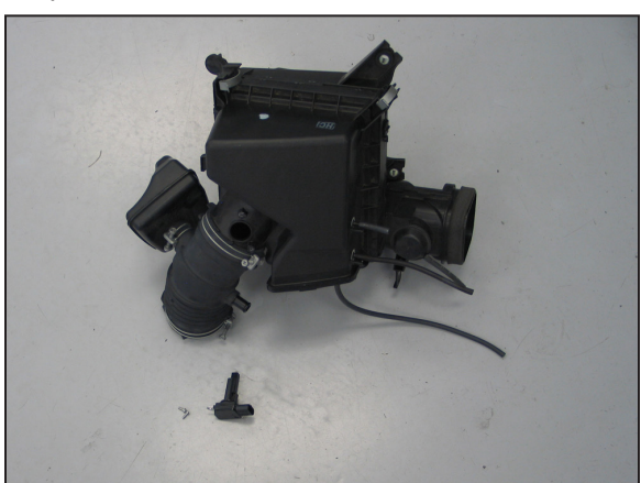
30. Remove the two screws securing the mass air sensor and then remove the mass air sensor from the factory air box.
