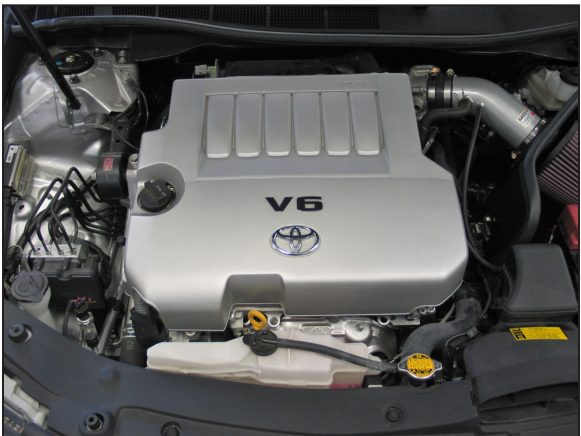
42. Install the engine cover.
