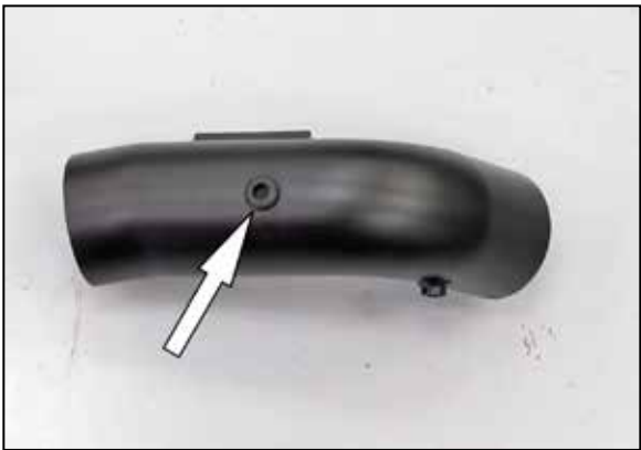
23. Install the provided grommet into the K&N® intake tube as shown.
