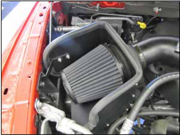
30. Install the K&N® air filter and secure with the provided hose clamp.
