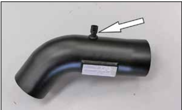
26. Install the inlet air temperature sensor into the grommet installed into the K&N® intake tube as shown.
