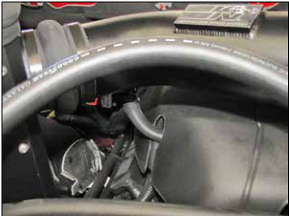
28. Connect the crank case vent hose to the fitting installed into the K&N® intake tube and secure with the provided hose clamp.
