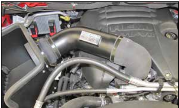
27. Install the K&N® intake tube into the silicone hump hose and then align with the hose on the throttle body. Align the hose, tube and heat shield for proper fit and then secure with the provided hardware.
