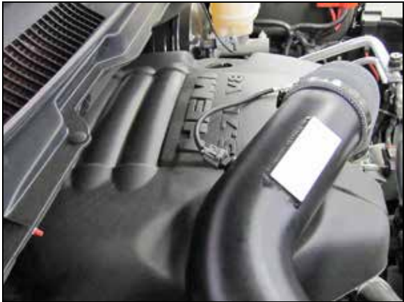
29. Choose the appropriate inlet air temperature sensor extension harness and then connect Install it too the inlet air temperature sensor and vehicle harness.
