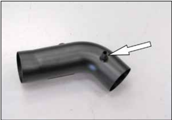
24. Install the vent fitting into the K&N® intake tube as shown.
