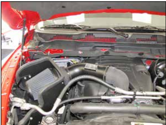
31. Reconnect the vehicle's negative battery cable. Double check to make sure everything is tight and properly positioned before starting the vehicle.
