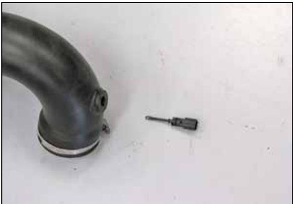
25. Remove the inlet air temperature sensor from the factory intake tube as shown.
