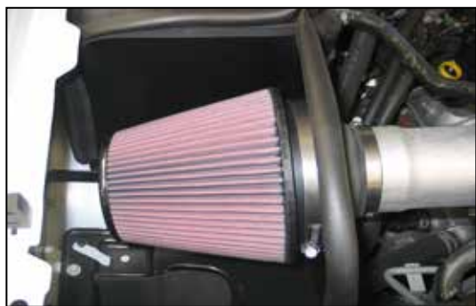
26. Install the K&N® air filter onto the filter adaptor and secure with the provided hose clamp. NOTE: Drycharger® air filter wrap; part # RF-1042DK is available to purchase separately. To learn more about Drycharger® filter wraps or look up color availability please visit http://www.knfilters.com ®.
