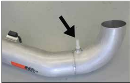
23. Install the provided 1/4" NPT fitting into the K&N® intake tube as shown. NOTE: Plastic NPT fittings are easy to cross thread. Install the vent fitting "hand" tight, then turn it two complete turns with a wrench.
