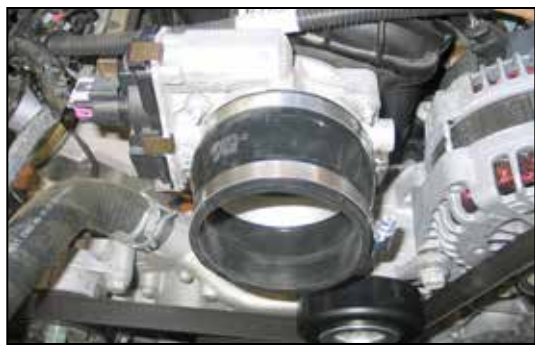
22. Install silicone hose (#08050) onto the throttle body and secure with the provided hose clamp.
