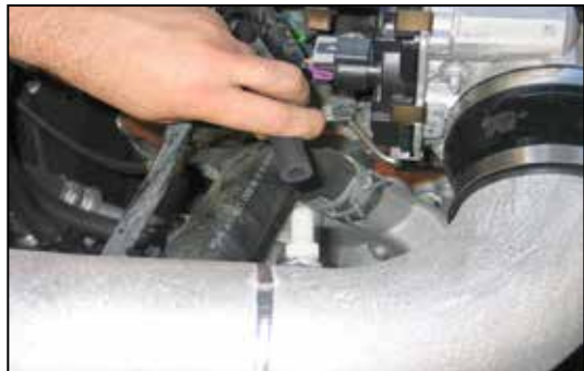
25. Install the provided crank case vent hose onto the valve cover vent port and then connect the remaining open end to the 1/4" NPT fitting in the K&N® intake tube.
