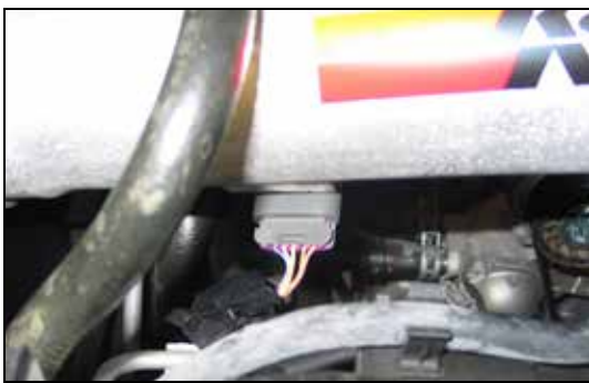
27. Reconnect the mass air electrical connection.
