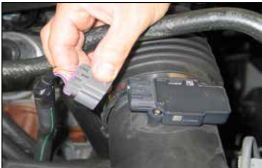
2. Disconnect the mass air electrical connection.
