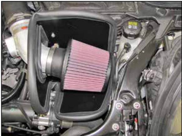
16. Install the K&N® air filter onto the intake tube and secure with the provided hose clamp. Adjust the tube and filter position for best fit.
