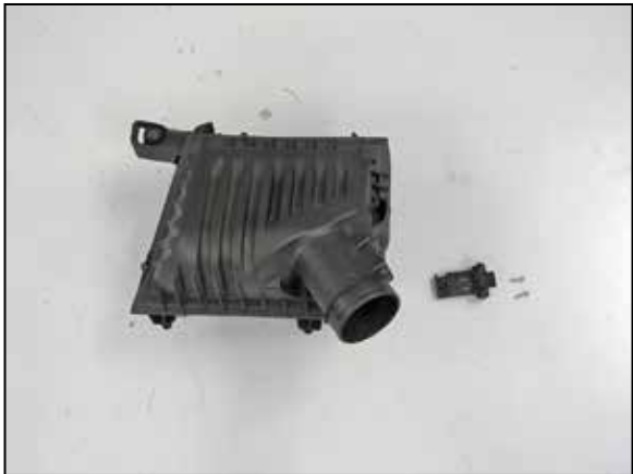
13. Remove the two bolts that secure the mass air sensor to the factory air filter housing and then remove the mass air sensor.
