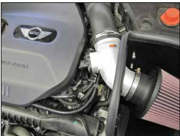
17. Reconnect the mass air sensor electrical connection.
