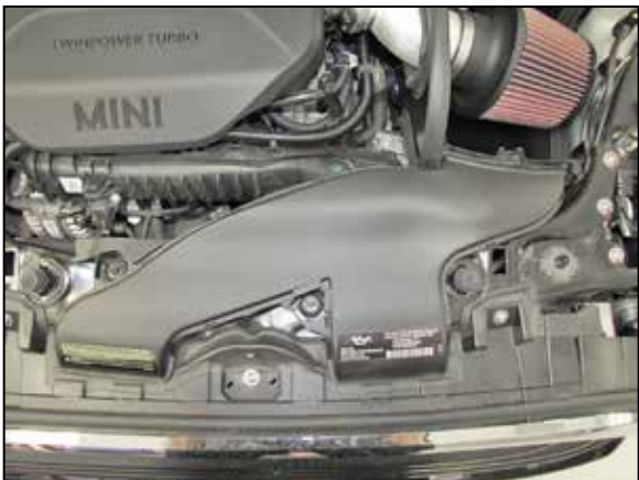
18. Reinstall the fresh air intake scoop and secure with the factory hardware.
