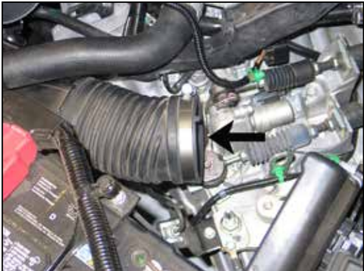
24. Install the provided hose clamp onto the stock fresh air supply hose as shown.
