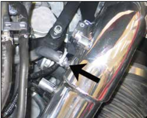
26. Install the EVAP hose onto the K&N® intake tube and secure it with the factory hose clamp.
