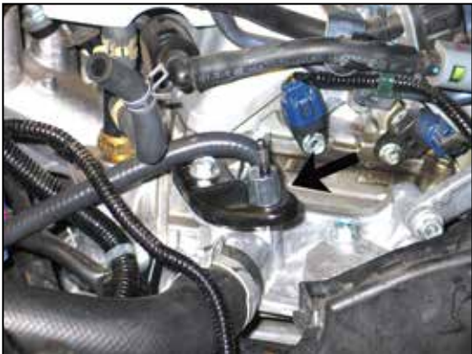
23. Install the provided spacer onto the airbox mounting stud as shown.
