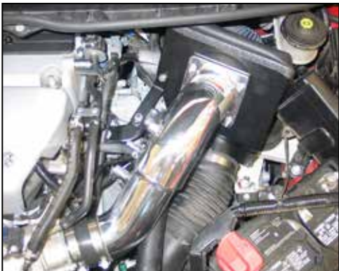
25. Install the intake assembly into the silicone hose at the throttle body and align the mounting bracket with the airbox mounting stud. Secure the intake assembly with the provided hose clamp and the factory nut that was removed in step #6. Secure the fresh air tube to the heat shield with the hose clamp.
