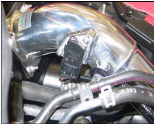
30. Re-connect the mass air sensor electrical connection.
