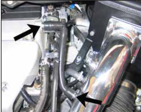
29. Install the crankcase vent hose assembly onto the valve cover port and intake tube port as shown.
