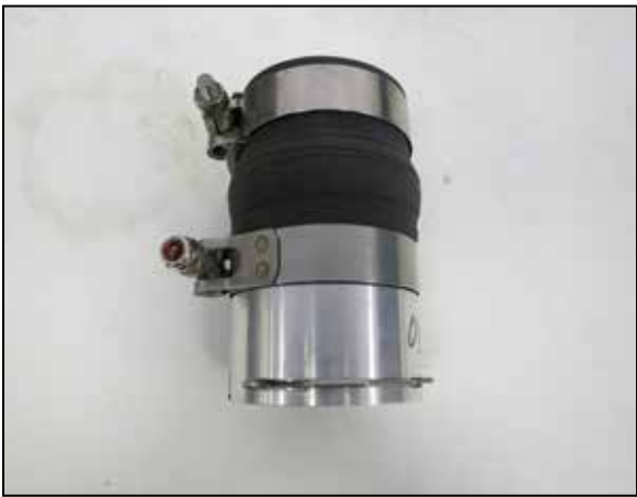
8. Install the hump coupler onto the K&N “Hot Side” inter cooler quick connector 088120 and secure with the provided hose clamp.
