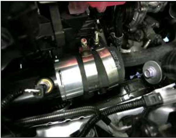
13. Install the “Cold Side” quick connector assembly onto the inter cooler outlet. Push the coupler onto the inter cooler until an audible “click” is heard as the retaining clip locks onto the inter cooler outlet.
