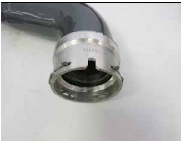
7. Remove the retaining clip and O-ring from the engine side of the factory “Hot Side” charge tube and install them into the “Hot Side” K&N charge tube. NOTE: notice the direction the lip is pointed on the O-ring and be sure to position the same direction in the K&N coupler.
