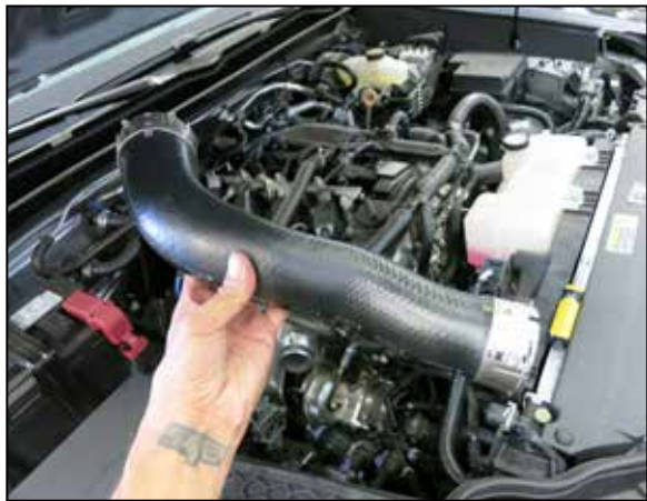
5. Release the retaining clips on the “Hot Side” charge tube in the same manner as the “Cold Side” and then remove the “Hot Side” charge tube from the vehicle.
