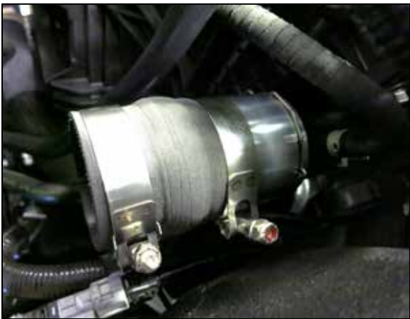
9. Install the “Hot Side” quick connector assembly onto the inter cooler as shown. Push the coupler onto the inter cooler until an audible “click” is heard as the retaining clip locks onto the inter cooler inlet.
