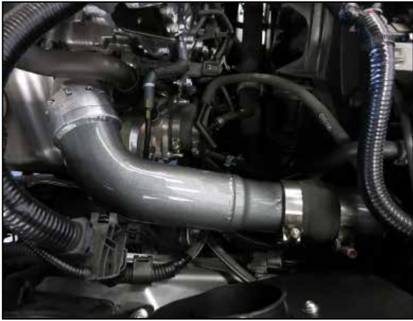
10. Install the K&N “Hot Side” charge tube into the coupler, then position the tube onto the turbo outlet and push the tube onto the outlet until an audible “click” is heard as the retaining clip locks onto the outlet. Position the tube and coupler for best fit and then secure the hose clamps.
