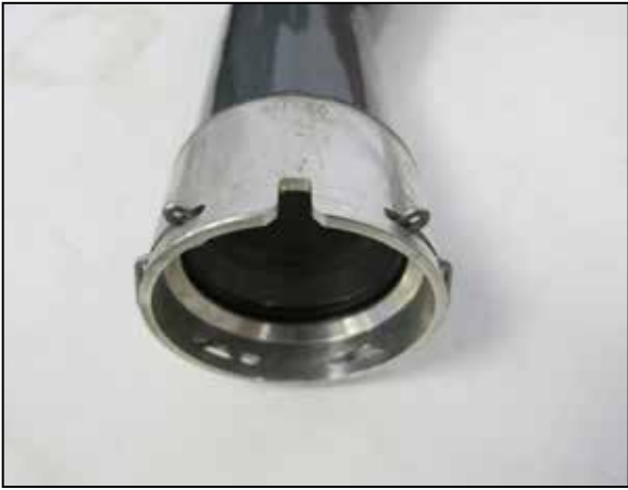
11. Remove the O-rings and retaining clips from the “Cold Side” charge tube and install them into the K&N “Cold Side” charge tube and quick coupler 088121. NOTE: notice the direction the lip is pointed on the O-ring and be sure to position the same direction in the K&N coupler.
