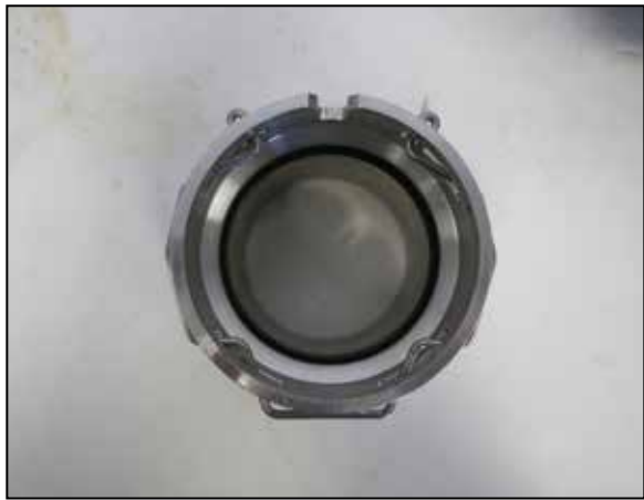
6. Remove the retaining clip and O-ring from the inter cooler side of the “Hot Side” charge tube and install them into the K&N “Hot Side” Charge tube inter cooler quick coupler 088120 as shown. NOTE: notice the direction the lip is pointed on the O-ring and be sure to position the same direction in the K&N coupler.
