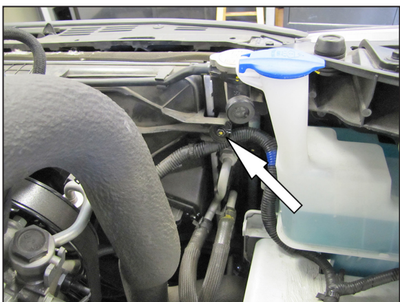
15. Remove the upper, right fan shroud mounting bolt shown.
