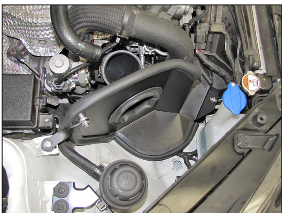
16. Install the heat shield assembly into the vehicle and secure to the rubber mounted stud and fan shroud using the provided hardware.
