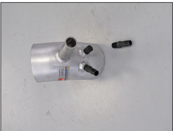
17. Install the provided fittings into the K&N® intake tube as shown. NOTE: On models equipped with a manual transmission, it will be necessary to install two vent fittings. NOTE: Plastic NPT fittings are easy to cross thread. Install the vent fitting "hand" tight, then turn it two complete turns with a wrench.
