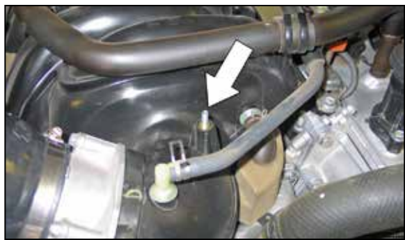
27. Install the provided stud into the mounting stud location as shown.
