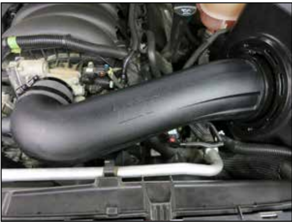
19. Install the intake tube to vehicle and position to air filter and hose on throttle body.
