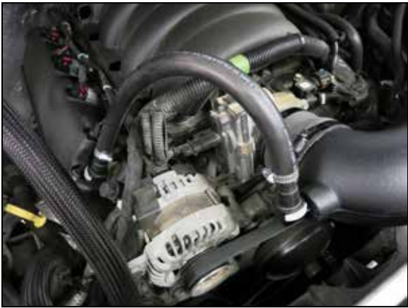
21. Install the crank case hose to the engine and intake tube, make sure you hear the click on the PCV connector.
