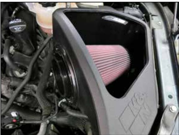
17. Install the air filter into the K&N airbox.
