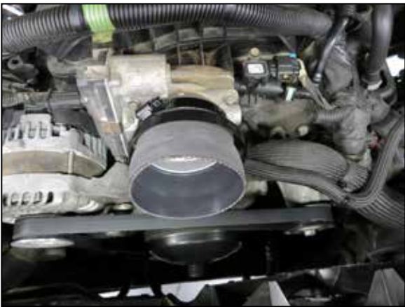
18. Install the 08497 hose to the throttle body with clamps provided for 5.3L models. Install the 084107 hose for the 6.2L models.
