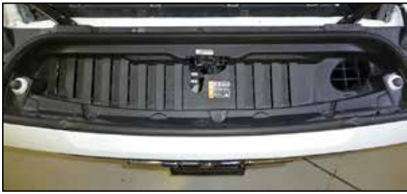
23. Reinstall the radiator valence and secure with the ten factory clips.
