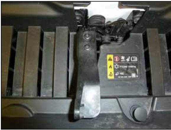
24. Reinstall the hood release arm and secure with the factory hardware.
