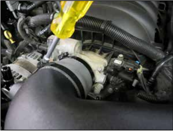
20. Adjust for proper fit, and tighten all clamps.
