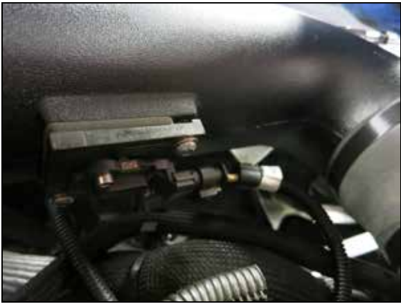
22. Connect the MAF sensor using provided harness extension, and secure harness using cable tie.
