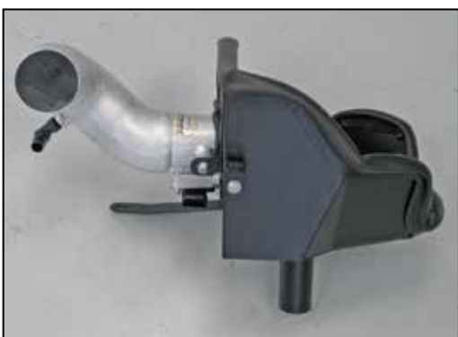
24. Install the K&N intake tube into the heat shield and secure to the mounting bracket with the provided hardware.
