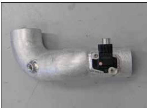
17. Install the mass air sensor into the K&N intake tube and secure with the provided hardware.
