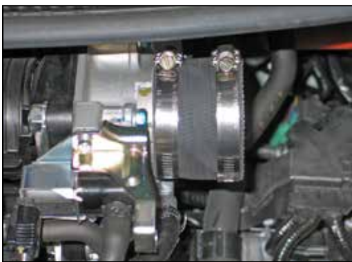
15. Install the provided silicone hose (08284) onto the throttle body and secure with the provided hose clamp.
