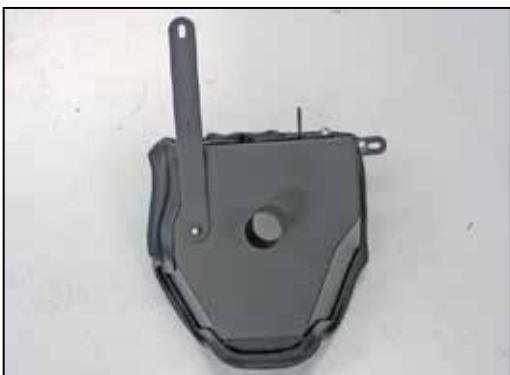
23. Install the flat bracket (083148) onto the heat shield as shown using the provided hardware.
