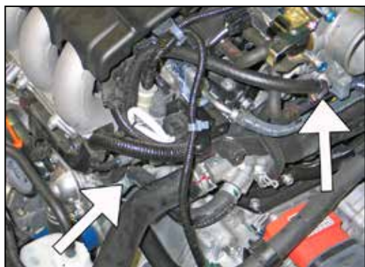
14. Remove the cap plugs and install the bypass hose onto the coolant fittings and secure with the provided hose clamps. NOTE: Be sure to replenish the captured coolant into the reservoir.
