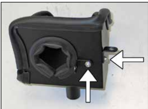
22. Install the provided "L" brackets (070066) onto the heat shield as shown using the provided hardware.
