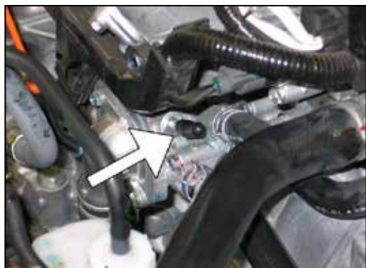
12. Release the spring clamp securing the coolant bypass hose to the thermostat housing. Remove the bypass hose from the thermostat housing fitting, quickly plugging the outlet with the remaining cap plug to prevent coolant loss. Remove the bypass/crankcase vent hose assembly from the vehicle. NOTE: Be sure to capture any released coolant.
