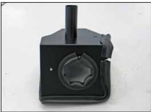
21. Install the 11" long edge trim into the hole of the heat shield.
