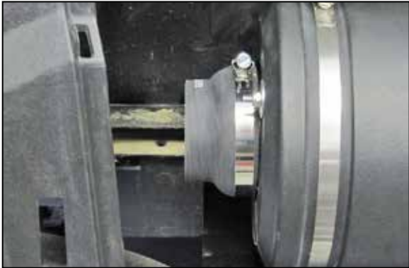
18. Install the provided coupler hose (084093) onto the filter adapter and secure with the provided hose clamp.
