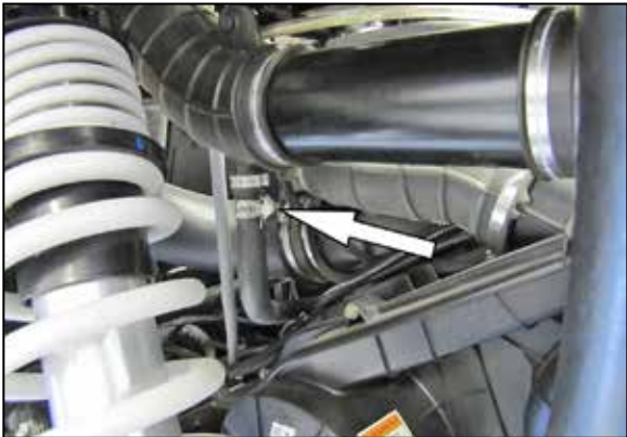
7. Loosen the clamp securing the vent hose to the intake tube.
