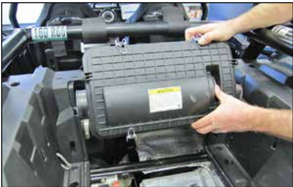
6. Remove the air filter housing from the vehicle. NOTE: K&N Engineering, Inc., recommends that customers do not discard factory air intake.
