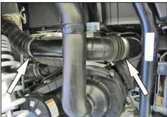
8. Loosen the hose clamp at the plenum and remove the bolt securing the intake tube. Then remove the intake tube from the vehicle.
