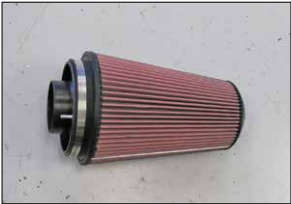
14. Install the adapter assembly into the K&N® air filter and secure with the provided hose clamp.
