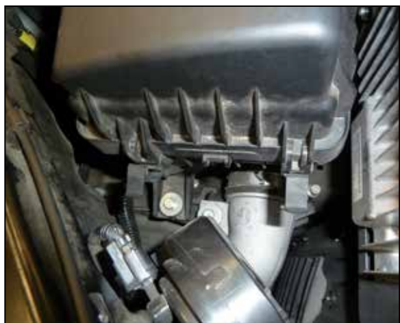
5. Release the two spring clamps that secure the air filter housing lid, remove the lit, intake hose and factory air filter.
