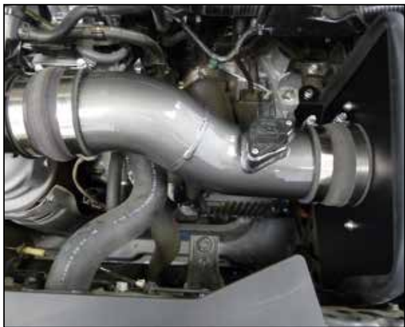
14. Install the K&N intake tube into the couplers, adjust for best fit and then secure with the provided hose clamps.
