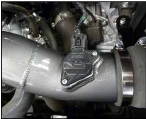
15. Reconnect the mass air sensor electrical connection.
