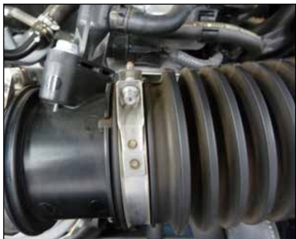
4. Loosen the clamp the secures the factory intake hose to the turbo inlet manifold.
