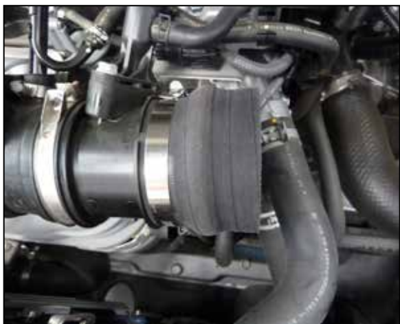
12. Install the provided hump coupler onto the turbo inlet manifold and secure with the provided hose clamp.
