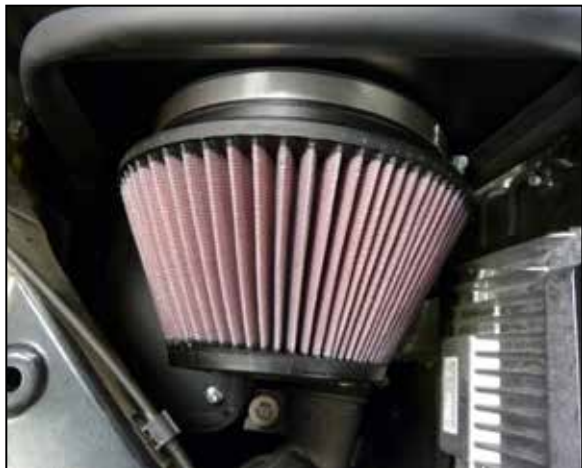
16. Install the K&N air filter and secure with the provided hose clamp.
