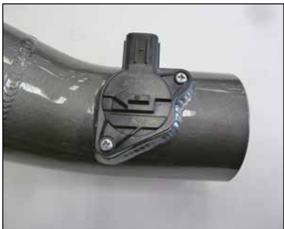
13. Remove the mass air sensor from the factory housing and install it into the K&N intake tube and secure with the factory mounting bolts.
