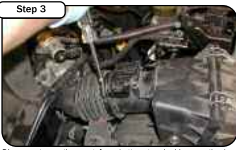
Disconnect negative post from battery terminal. Loosen the hose clamp on the intake duct. Disconnect the MAF sensor by pushing down on the clip and pulling out.
