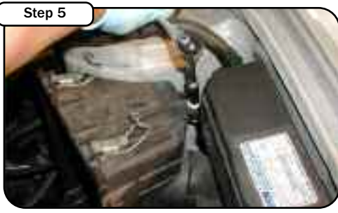
Remove the 10mm bolt that supports the other half of the airbox and remove the rest of the airbox.
