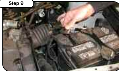
Reconnect the MAF sensor and tighten down the hose clamp on the intake pipe
