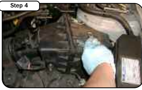
Unclip the two mounting clips located on the side of the airbox. Lift the top half of the airbox out and remove.
