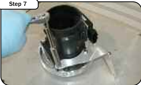
Bolt the MAF sensor to the billet adaptor using the supplied M6 screws and washers. On the right side of the sensor place the aluminum bracket and fasten to assembly as shown in photo.
