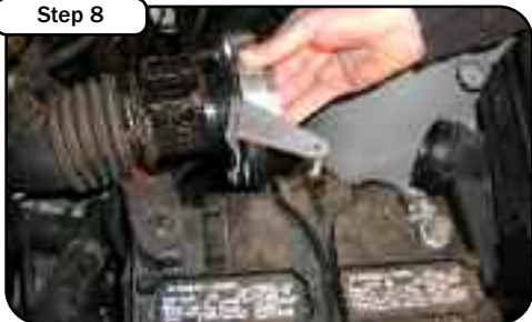
Remove the 10mm bolt supporting the battery strap. Position the intake assembly into the engine bay. Line up the hole on the bracket with the battery bracket as shown, reinstall bolt and tighten bolt to secure assembly.
