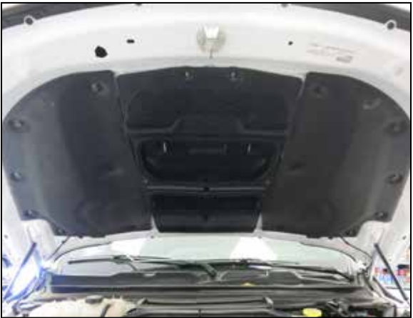
46. Reinstall the under hood insulation and secure with the provided retaining clips.
