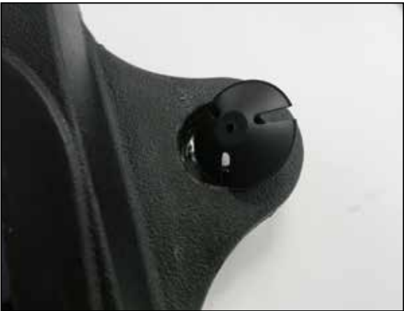
42. Feed two of provided retaining clips into the K&N fresh air duct as shown.
