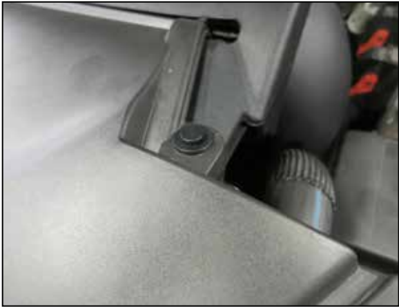
39. Install two provided retaining clips into the front into the front of the air filter housing through the valence.
