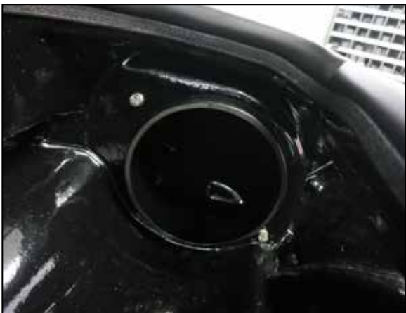
32. Position the intake tube into the air filter housing and then secure the tube to the housing with the provided hardware.
