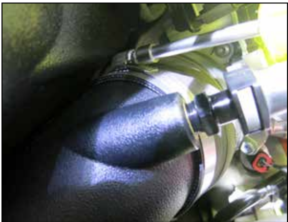
35. Tighten the hose clamp that secures the K&N intake tube to the coupler at the throttle body.
