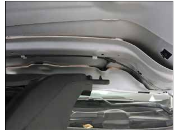
44. Rotate the fresh air duct up and align the mounting clips previously installed to the mounting holes in the hood.
