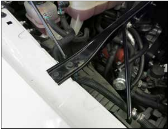
33. Secure the front air filter housing mounting bracket to the core support using the factory air filter housing mounting bolts.
