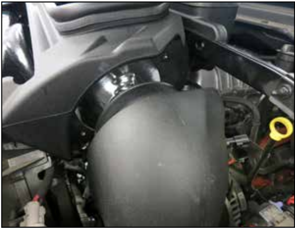
31. Set the air filter housing assembly into the vehicle.
