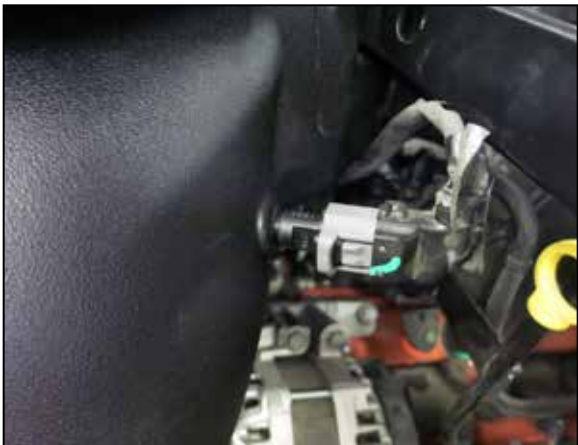
36. Reconnect the IAT sensor electrical connection.
