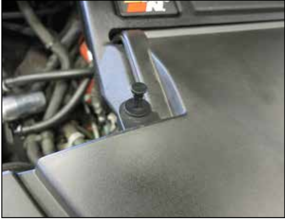
38. Reinstall the upper valence and secure with the factory retaining clips.
