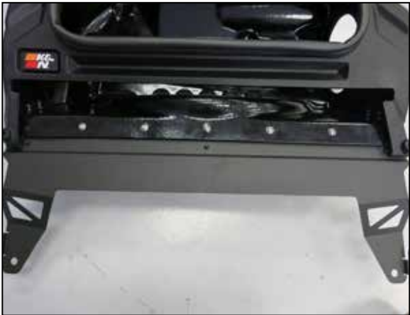
30. Secure the top side of the filter housing to the support bracket with the provided hardware.
