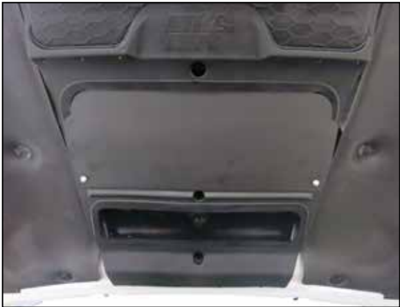
47. During severe inclement weather such as heavy rain or snow, K&N recommends install the provided forward fresh air block off plate using the provided hardware.
