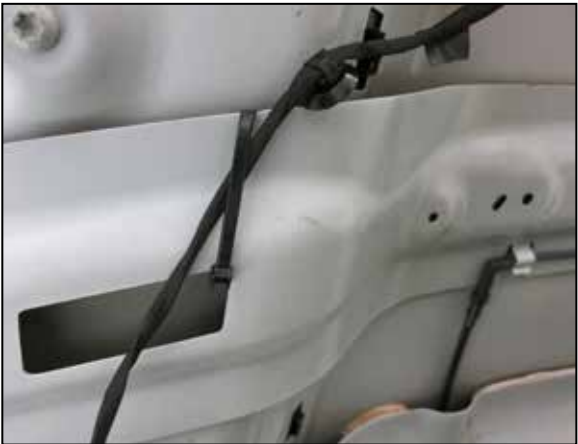
41. Using the provided tie wrap, secure the harness to the hood as shown.
