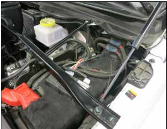
34. Secure the air filter support bracket onto the inner fenders using the factory hardware.
