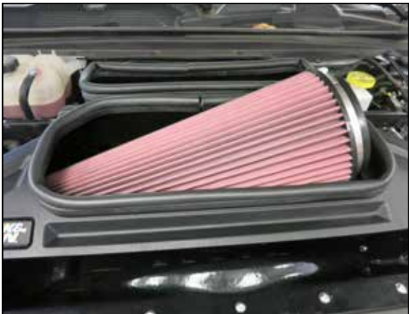
37. Install the K&N air filter into the housing and onto the intake tube, then secure with provided hose clamp.
