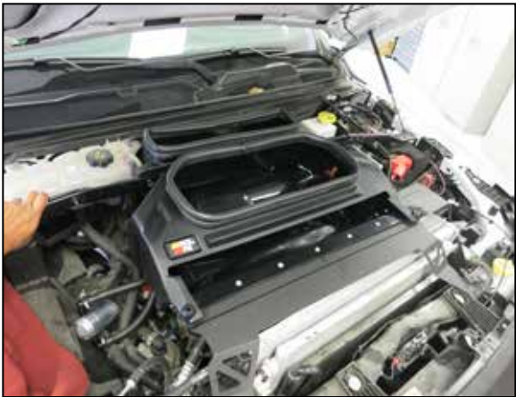
31. Set the air filter housing assembly into the vehicle.
