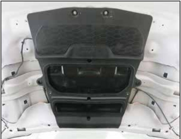
45. Snap the retaining clips into the hood and then secure the front of the duct to the hood with the hardware provided.
