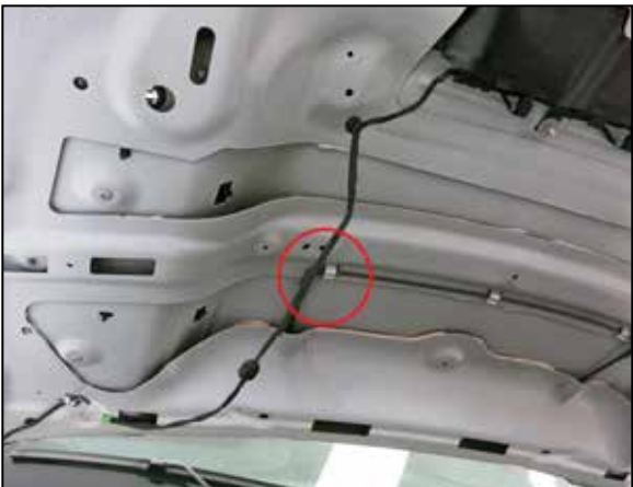
40. Unclip the wiring harness from the under side of the hood where shown.
