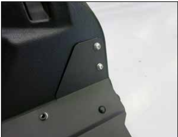
29. Secure the support bracket to the K&N air filter housing with the provided hardware.
