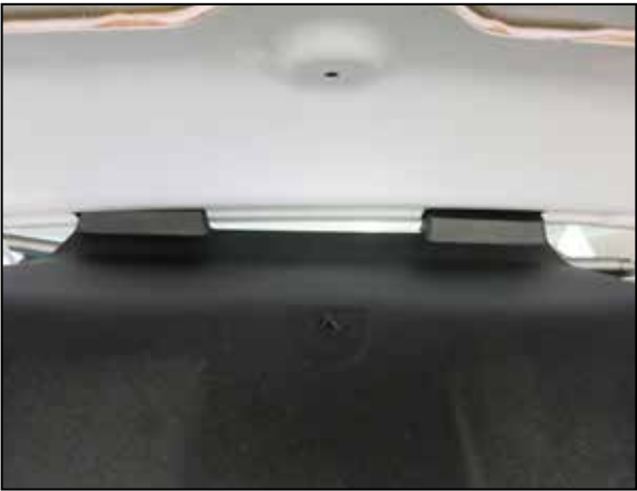
43. Install the tabs at the rear of the K&N fresh air duct onto the slots of the hood.
