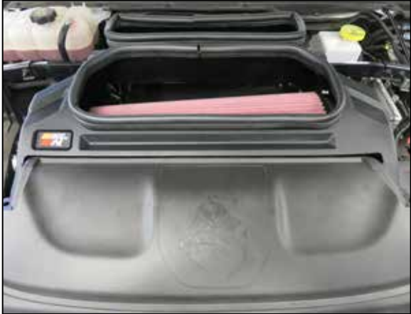
38. Reinstall the upper valence and secure with the factory retaining clips.
