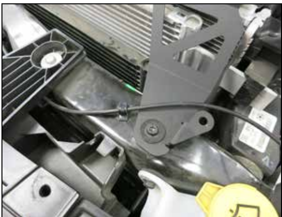
33. Secure the front air filter housing mounting bracket to the core support using the factory air filter housing mounting bolts.
