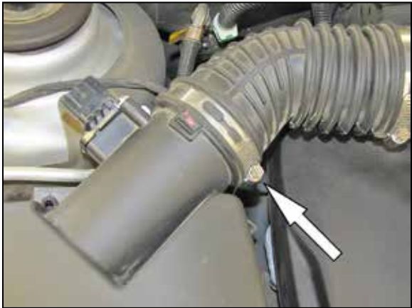
4. Loosen the hose clamp securing the intake tube to the air filter housing.
