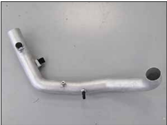
18. Install the 90° npt fitting into the K&N intake tube as shown.
