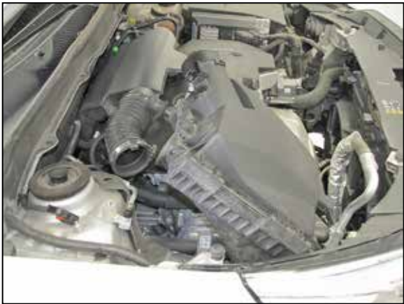
5. Lift up the rear of the air box so that it becomes disengaged with the mounting grommet saddle, and then remove the complete air box from the vehicle. NOTE: K&N Engineering, Inc., recommends that customers do not discard factory air intake.
