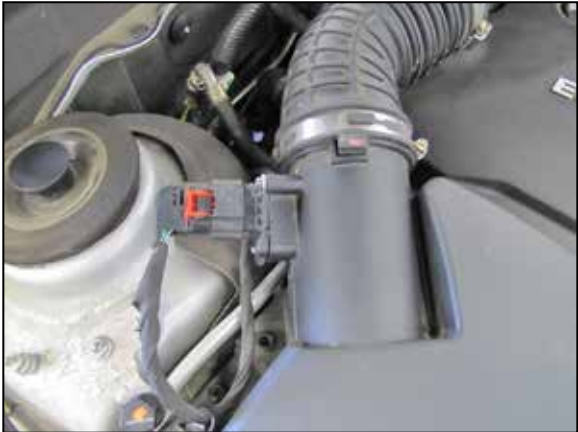
2. Disconnect the mass air sensor electrical connection.
