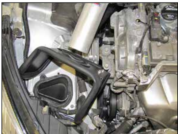
27. Set the heat shield onto the engine mount so the bracket lines up with the engine mounting bolt hole. Reinstall the engine mounting bolt.
