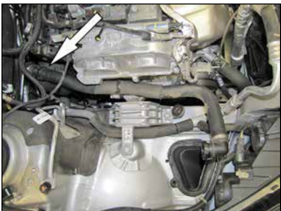
12. On vehicles equipped with air injection, cut the clamp at the air injection hose union and then separate the air injection hose and remove the loose section from the vehicle.
