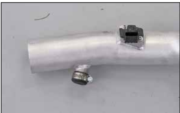
17. On vehicles that are not equipped with air injection, install the provided cap plug onto the air injection port and secure with the provided hose clamp.
