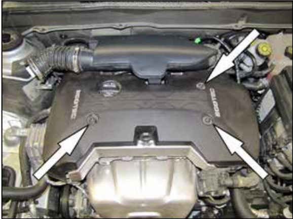
6. Remove the three screws securing the engine cover, remove the oil cap and then remove the engine cover. Reinstall the oil cap for now to prevent debris from entering the engine.
