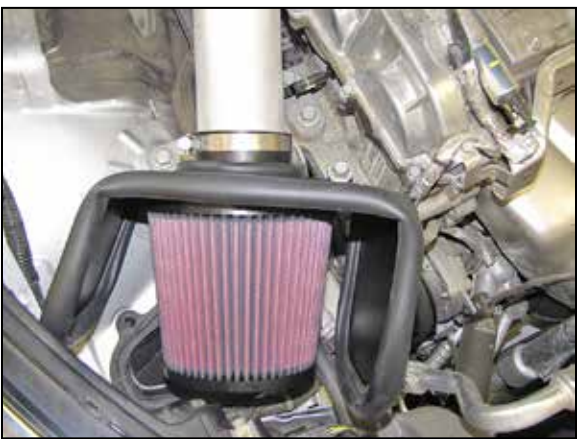
28. Install the K&N® air filter and secure with the provided hose clamp. NOTE: Drycharger® air filter wrap; part # RX-4990DK is available to purchase separately. To learn more about Drycharger® filter wraps or look up color availability please visit http://www.knfilters.com ®.
