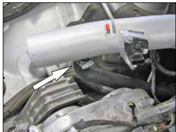
22. On vehicles equipped with air injection, connect the hose to the fitting in the intake tube and secure with the provided hose clamp.
