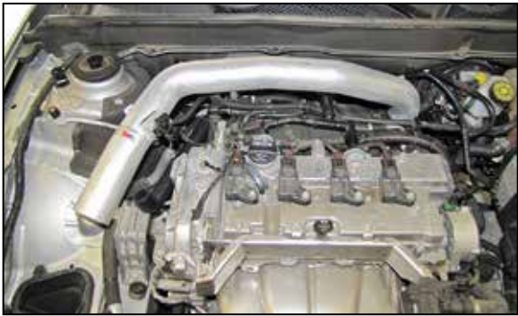
21. Install the K&N intake tube into the coupler on the throttle body and align with the plenum mounting bracket. Secure the intake tube with the provided hardware and hose clamp. Install the provided crank case vent hose onto the fitting installed onto the K&N intake tube, then attach the hose to the factory crank case vent assembly and connect it to the factory fittings on the valve cover. NOTE: Some trimming of the provided hose may be necessary to prevent the hose from pinching.
