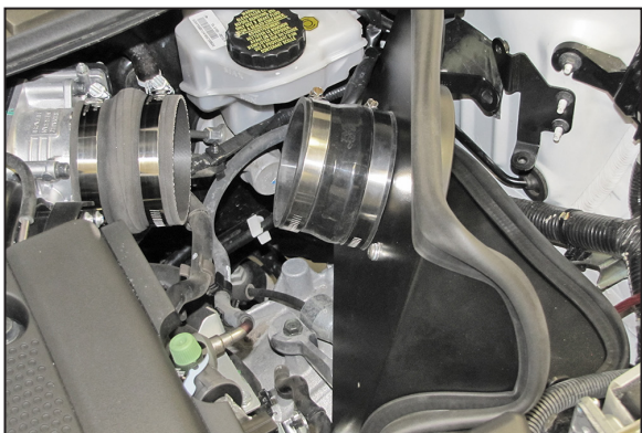
16. Install the provided coupling hose (08051) onto the filter adapter and secure with the provided hose clamp.
