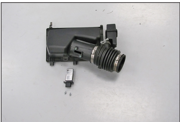
17. Remove the mass air sensor from factory air box.
