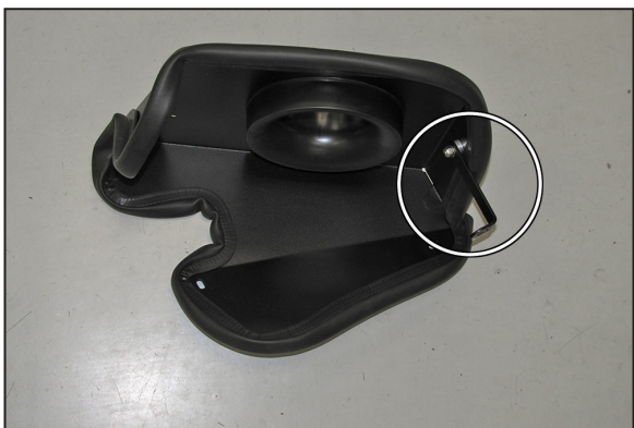
12. THIS STEP IS FOR THE NISSAN ALTIMA, FOR NISSAN PATHFINDER AND INFINTI JX35 VEHICLES, SKIP TO STEP #13. Install the provided heat shield mounting bracket (010040) onto the heat shield as shown. Be sure to use the provided spacer between the bracket and heat shield.
