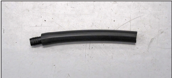
21. Install the hose mender into the provided crank case vent hose as shown.
