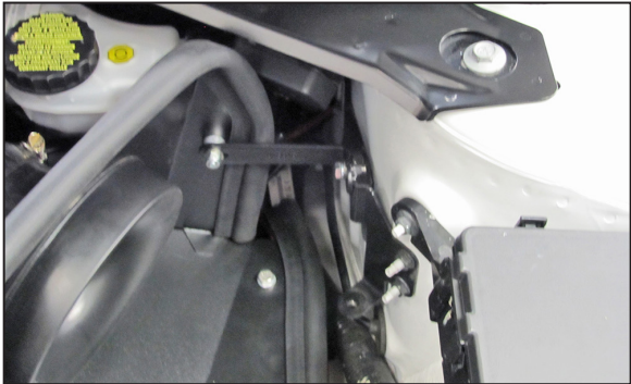
20. Secure the heat shield mounting bracket to the air box bracket on the strut tower with the provided hardware. NOTE: On Nissan Pathfinder and Infiniti JX35 vehicles, the mounting bracket will be secured to the rubber mounted stud installed during step #9.
