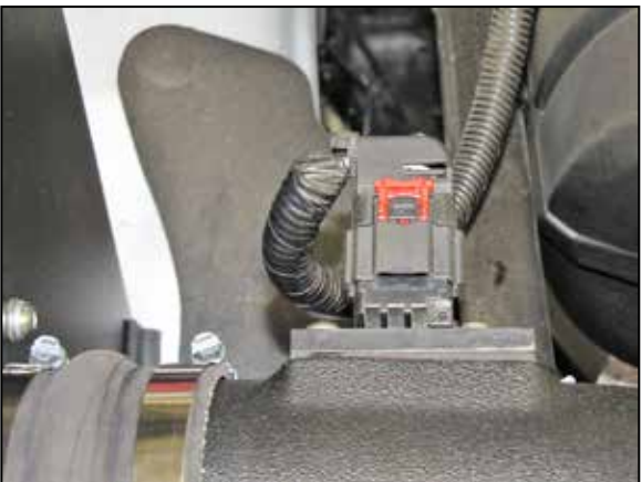
23. Reconnect the mass air sensor electrical connection.
