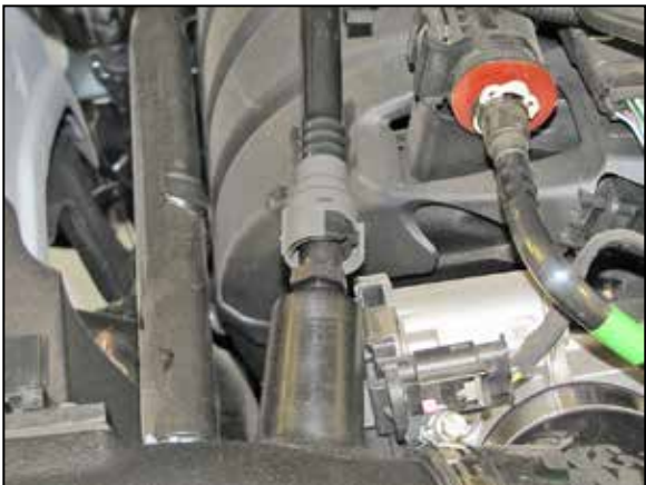
22. Connect the crank case vent hose to the fitting installed into the K&N® intake tube.
