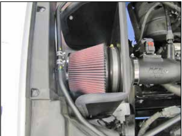
24. Install the K&N® air filter and secure with the provided hose clamp.
