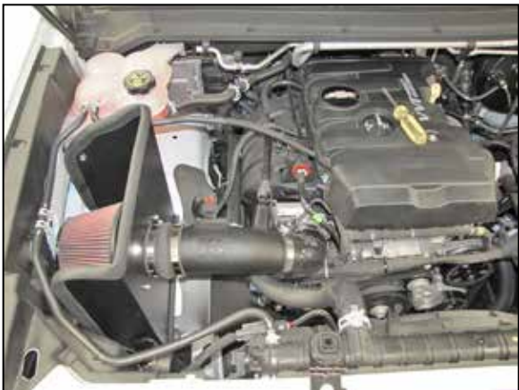
25. Reconnect the vehicle's negative battery cable. Double check to make sure everything is tight and properly positioned before starting the vehicle.
