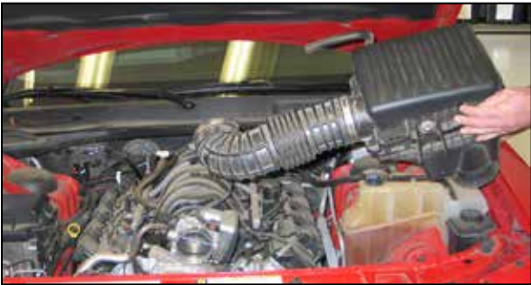
8. Lift and remove the complete intake assembly from the vehicle.
