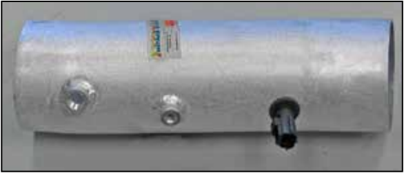
17. Install the inlet air temperature sensor into the grommet installed in the previous step.
