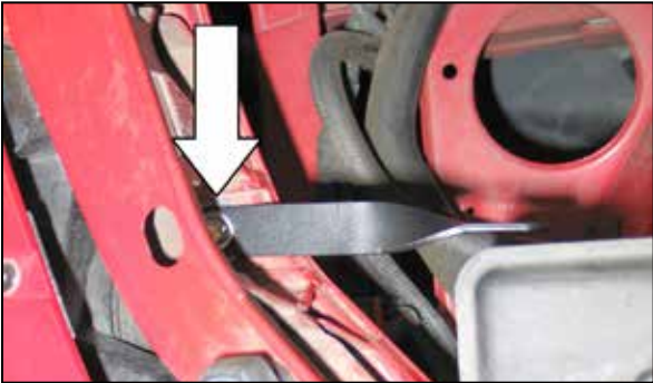
9. Install the twist bracket (070772) onto the core support using the provided hardware through the existing hole as shown.
