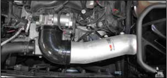
19. Install the K&N intake tube into the silicone hose at the throttle body and align with the heat shield and mounting bracket. Secure the intake tube with the hose clamp and hardware provided.
