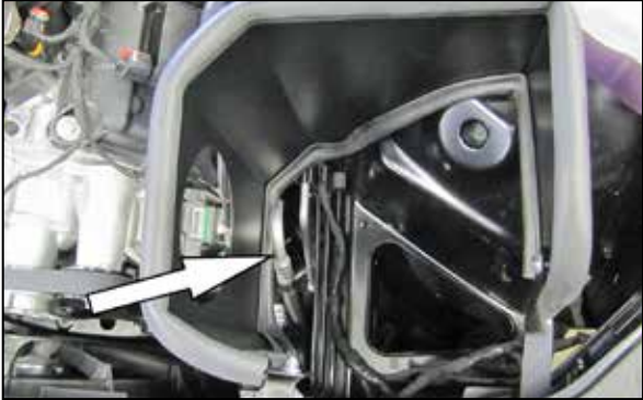
12. Install the heat shield assembly into the vehicle and secure to the bracket installed in step #9. Then secure the "L" bracket with the factory bolt removed in step #6 to the airbox mounting location.
