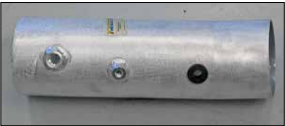
16. Install the provided grommet into the K&N intake tube as shown.
