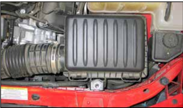
7. Loosen and remove the airbox mounting nut shown.
