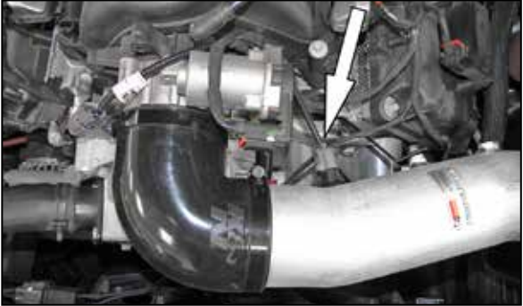
21. Connect the provided inlet air temperature sensor harness extension into the factory harness, run it under the throttle body and then connect to the inlet air temperature sensor as shown. Using the provided cable tie, secure the harness extension tube mounting bracket. NOTE: Inspect the inlet air temperature sensor to determine which of the two provided harnesses will be needed.
