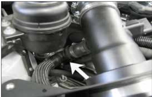
30. Route the air injection hose under the heat shield and connect to the silicone hose on the intake tube and secure with the provided hose clamp as shown.
