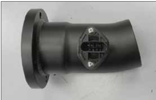
34. Install the mass air sensor into the left intake tube (27283) and secure with the provided hardware.
