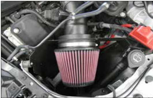
38. Install the air filter and secure with the provided hose clamp.
