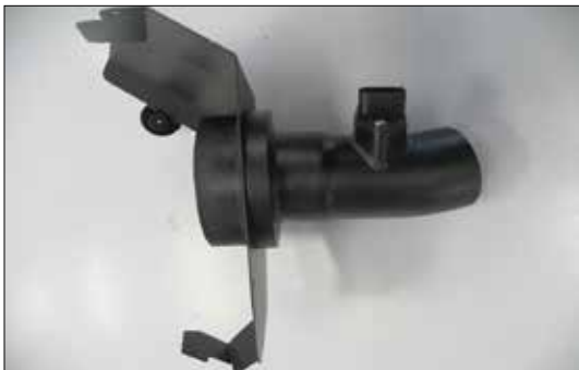
35. Assemble the left intake tube, heat shield, and filter adapter using the supplied gaskets and hardware. NOTE: Use two gaskets, one on either side of the heat shield between the filter adapter and intake tube.
