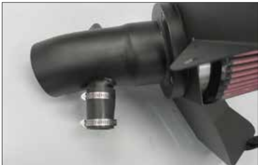
27. Install the provided air injection hose onto the intake tube and secure with the provided hose clamp as shown.
