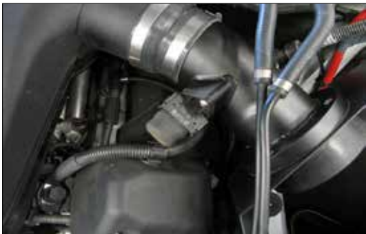
37. Reconnect the left mass air sensor electrical connection.
