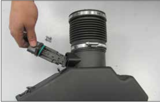
33. Remove the two screws that secure the left mass air sensor to the left upper air box and then remove the mass air sensor.
