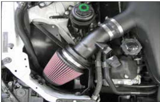
29. Install the right intake tube into the silicone hose on the intake plenum, align the grommet in the bottom hole of the heat shield with air box bumper stud on the inner fender and then secure the heat shield to the rubber mounted stud installed on the inner fender during step #20.
