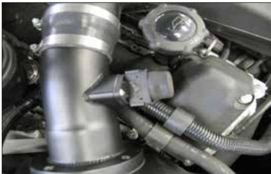
32. Reconnect the right mass air sensor electrical connection.
