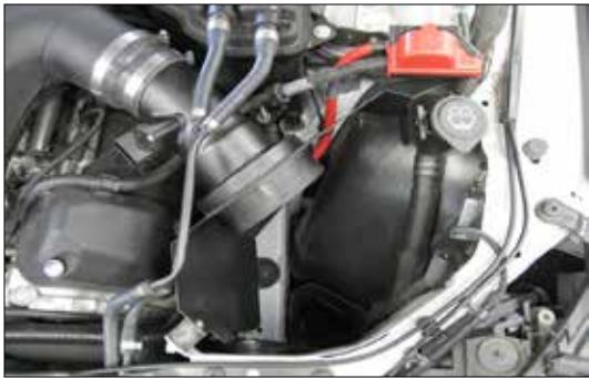
36. Install the left intake tube into the silicone hose on the intake plenum, align the grommet in the bottom hole of the heat shield with air box bumper stud on the inner fender and then secure the heat shield to the rubber mounted stud installed on the radiator core support during step #21. Note: Attach windshield washer fill hose to heat shield.
