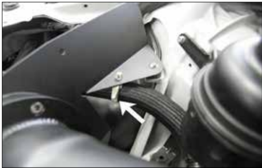
31. Install the supplied cable tie through the hole in the heat shield and then secure the air injection hose as shown.
