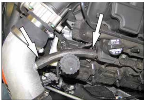
22. Install the provided crank case vent hose onto the valve cover port and then to the port on the K&N® intake tube. NOTE: Some trimming of the hose may be necessary.
