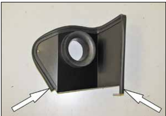
13. Install the edge trim onto the heat shield as shown. NOTE: Some trimming of the edge trim will be necessary.
