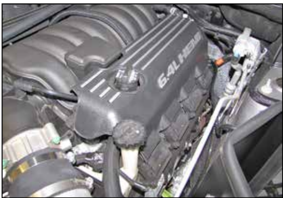
24. Reinstall the driver's side decorative engine cover.
