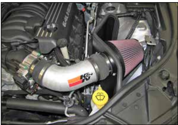
26. Reconnect the vehicle's negative battery cable. Double check to make sure everything is tight and properly positioned before starting the vehicle.
