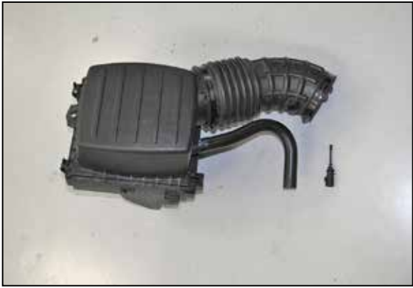
19. Remove the inlet air temperature sensor from the factory intake tube.
