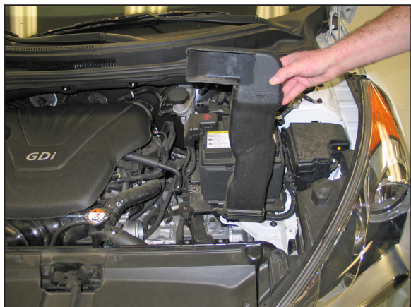
7. Remove the fresh air intake duct.
