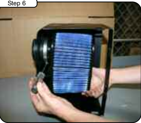
Insert and tighten your pre-oiled filter into the housing. Do not use any grease or oil.
