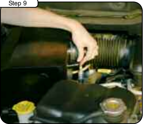
Re-connect your breather hose to the filter nipple. If your vehicle is not equipped with a breather hose, cap off the nipple with the supplied vacuum cap.
