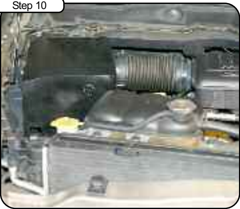
Place enclosed CARB EO sticker on a clean/smooth surface on or near the intake system. EO identification label is required to pass the smog inspection. Your installation is now complete. Tighten all connections and clamps. Re-check after a few hours.
