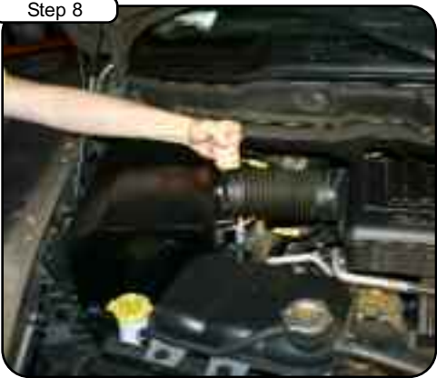
Re-connect air duct to the air filter housing. Tighten the factory hose clamp.
