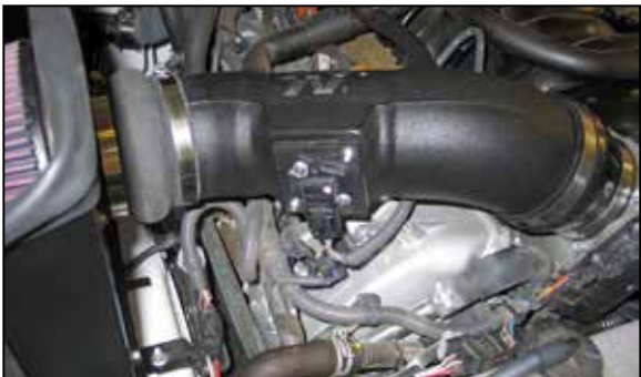
27. Reconnect the mass air sensor electrical connection.
