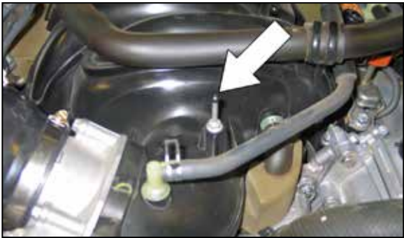
28. Remove the front engine cover mounting stud from the intake manifold.
