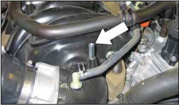
30. Install the provided nut extension onto the stud as shown.
