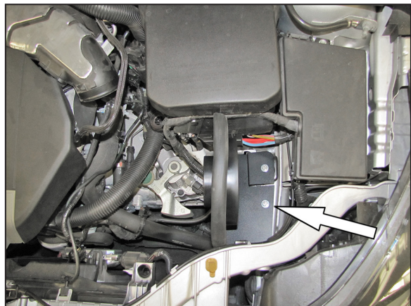
11. Install the heat shield assembly into the engine compartment and secure it to the rubber mounted stud with the provided hardware.
