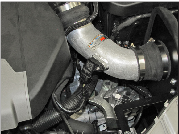
19. Reconnect the pressure sensor electrical connection.
