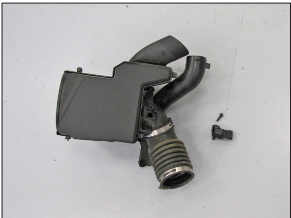
16. Remove the pressure sensor from the factory air box as shown.
