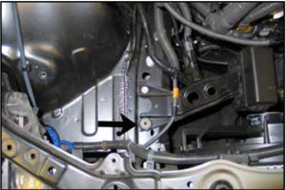
18. Install the rubber mounted stud into the relay mounting bracket as shown.
