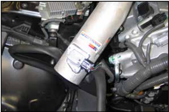
31. Using a small screw driver, remove the mass air sensor plastic elbow cover and then reconnect the mass air sensor electrical connection.
