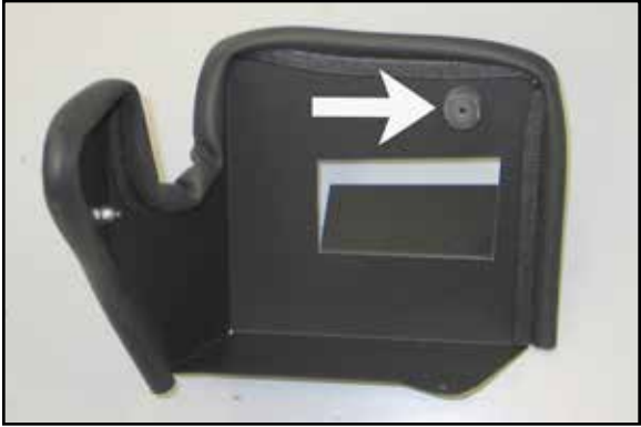
14. Install the rubber mounted stud onto the heat shield as shown.
