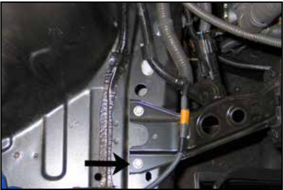
17. Remove the relay bracket mounting bolt shown.
