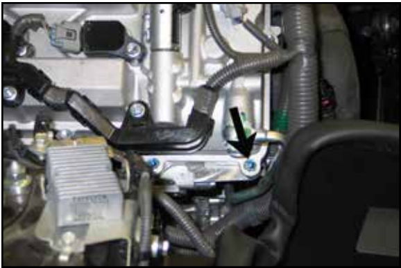
28. Remove the valve cover mounting bolt shown.
