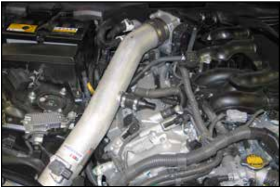
29. Install the K&N® intake tube into the silicone hose at the throttle body and align the bracket to the valve cover, secure with the factory valve cover bolt and hose clamp.
