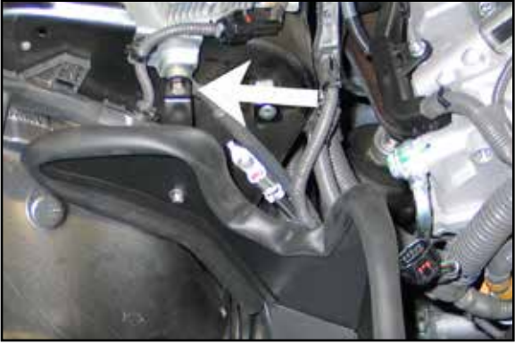
21. Set the heat shield into position and align with the rubber mounted stud, fender washer, and the ground strap bracket. Secure with provided hardware. NOTE: Be sure to use the provide spacer on top of the ground strap.
