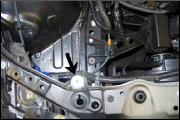
20. Install the fender washer and rubber washer onto the air box mounting point on the core support as shown.
