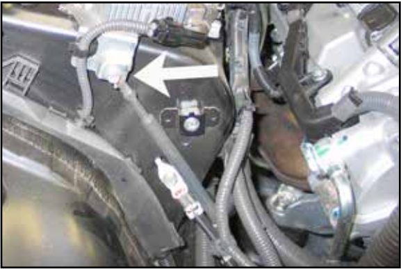
19. Remove the ground strap bolt shown.
