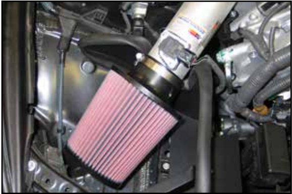
32. Install the K&N® air filter onto the intake tube and then tighten the hose clamp.
