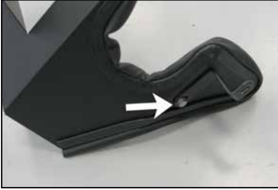
16. Install the “Z” bracket (020003) onto the heat shield as shown.
