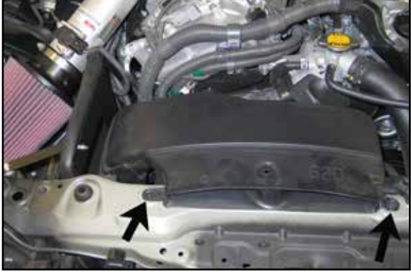
33. Reinstall the fresh air supply and secure with the factory bolt removed in step #6.
