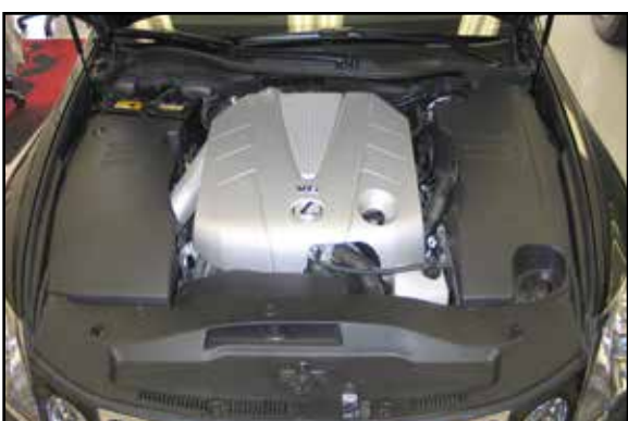
36. Reinstall the engine cover onto the top of the engine.
