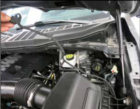
4. Disconnect the IAT sensor electrical connection and unhook the wiring harness from its mounts.
