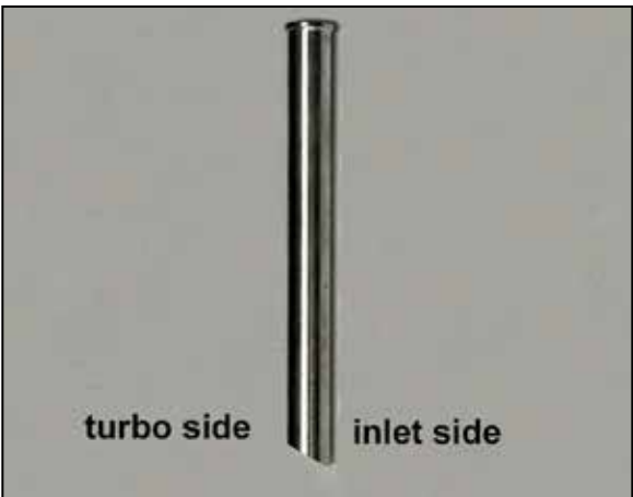
9. Install the provided CCV insert into the driver side inlet tube. NOTE: The Angled end of the cut needs to be installed with the shorter end towards the turbo and the longer end towards the inlet. Apply two drops of the provided superglue on the bottom of the lip of the insert before installation.
