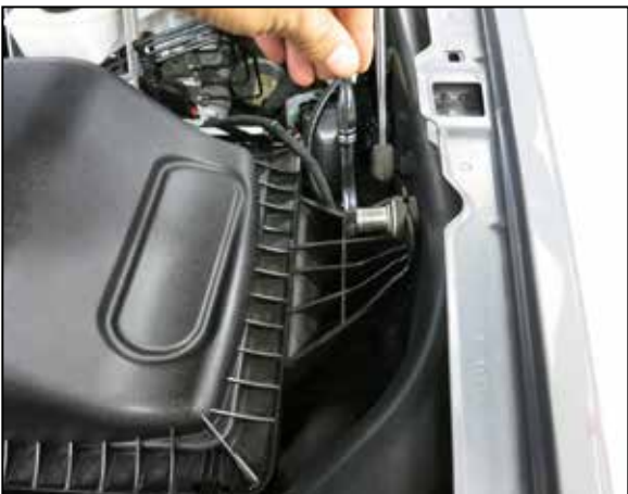
6. Remove the bolt that secures the factory air filter housing to the inner fender and then remove the air filter housing from the vehicle. This bolt will be reused in the next step.
