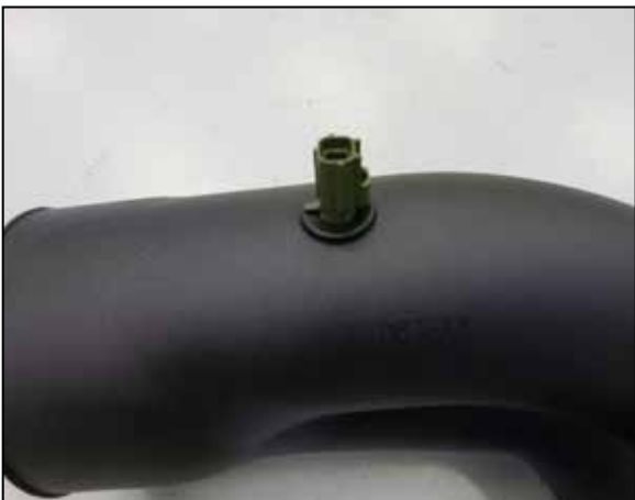
13. Remove the O-ring from the IAT sensor and then install the sensor into the K&N intake tube using the provided grommet.
