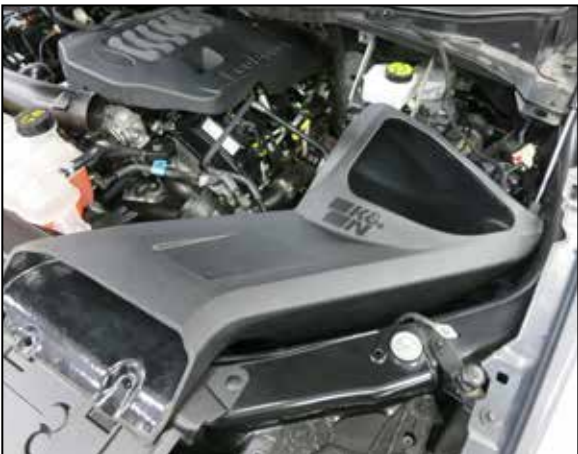
7. Install the K&N air filter housing and secure to the inner fender using the mounting bolt from the previous step.
