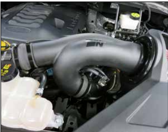
15. Install the K&N intake tube into the air filter and align with the turbo inlet tubes. Adjust the assembly for best fit and then tighten all the hose clamps.
