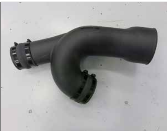
14. Install the provided couplers and clamps onto the K&N intake tube as shown but do not tighten the clamps.
