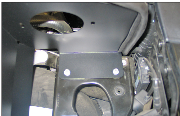
18. Reinstall the heat shield assembly onto the air box mounting plate and secure the two 5/16" bolts provided.
