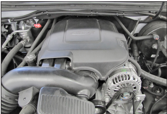
3. Lift up on the engine cover and remove as shown.
