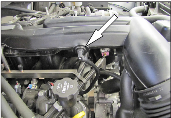
5. Unhook the crankcase vent line from the intake tube plenum as shown.
