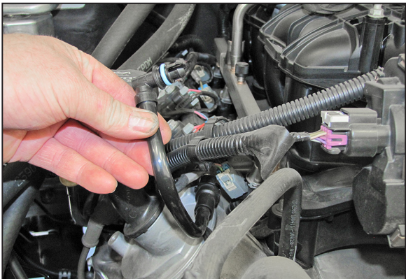
7. Rotate the crankcase vent line counter clockwise on the valve cover port, and then release the locking tab and remove the crankcase vent line from the valve cover.
