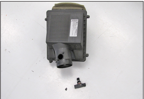
9. Remove the two screws securing the mass air sensor to the air box and then remove the mass air sensor from the air box as shown.
