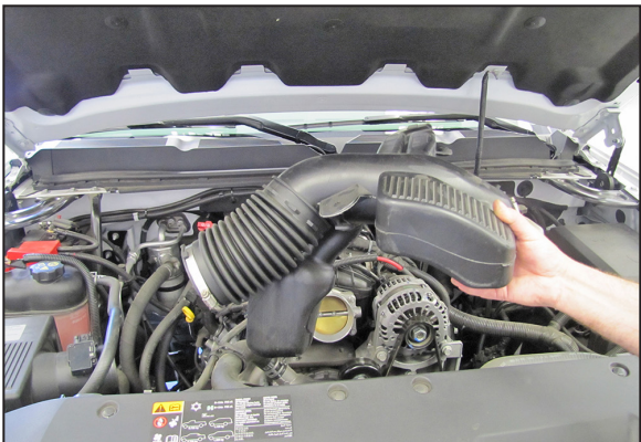
6. Loosen the hose clamps which secure the stock intake tube, then remove the intake tube from the vehicle.
