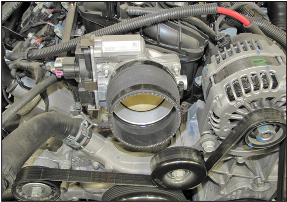
21. Install silicone hose (#08497) onto the throttle body and secure with the provided hose clamp.
