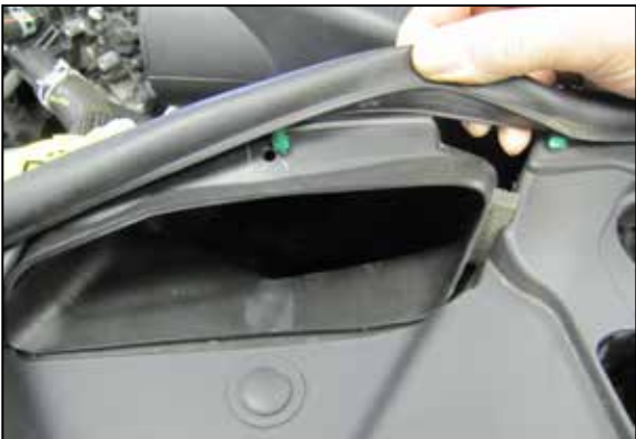
6. Unhook the hood seal mounting pin from the fresh air intake scoop.
