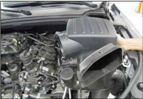
7. Lift the air filter housing to dislodge it from the mounting grommets and then remove it from the vehicle.
