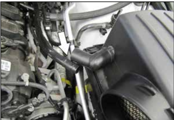
5. Disconnect the crank case vent tube from the elbow attached to the factory air filter housing as shown.
