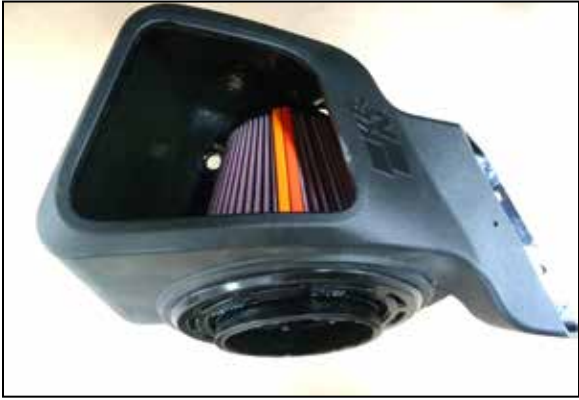
11. Install the K&N air filter into the K&N air filter housing as shown.
