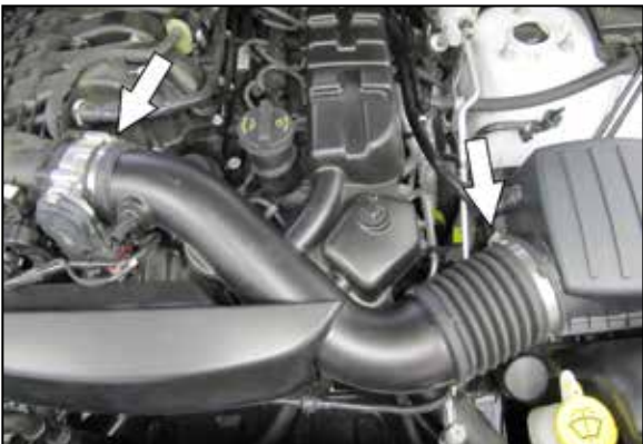
4. Loosen the hose clamps securing the intake tube to the throttle body and air filter housing and then remove the intake tube assembly from the vehicle. NOTE: The intake tube assembly is also held on with two mounting studs and grommets.
