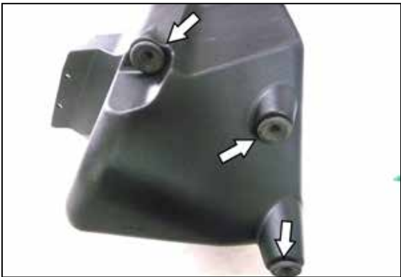
9. Install the three mounting grommets into the K&N air filter housing as shown.
