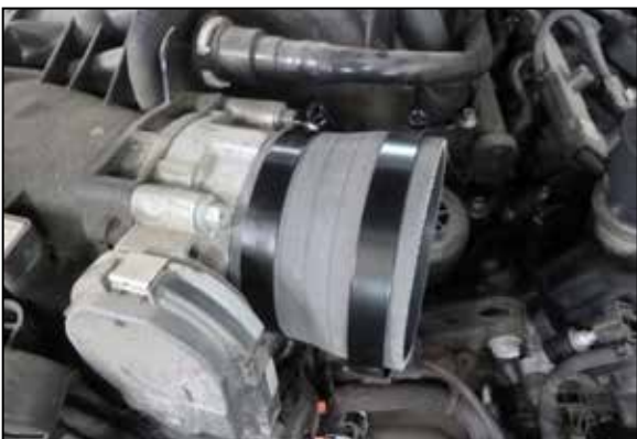
14. Install the provided coupler onto the throttle body and secure with the provided hose clamp.
