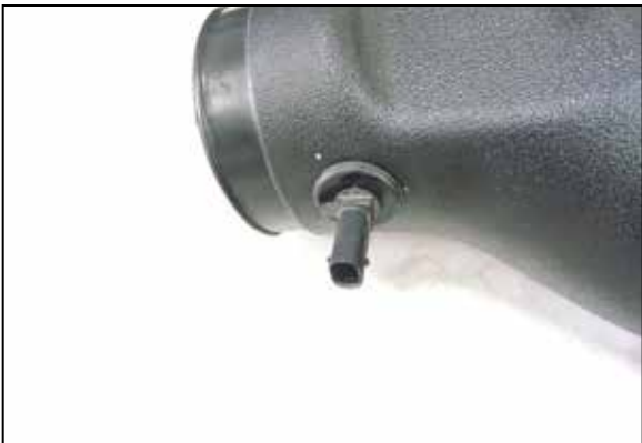
15. Remove the IAT sensor from the factory housing and remove the O-ring from the sensor. Install the sensor into the K&N intake tube using the provided grommet.
