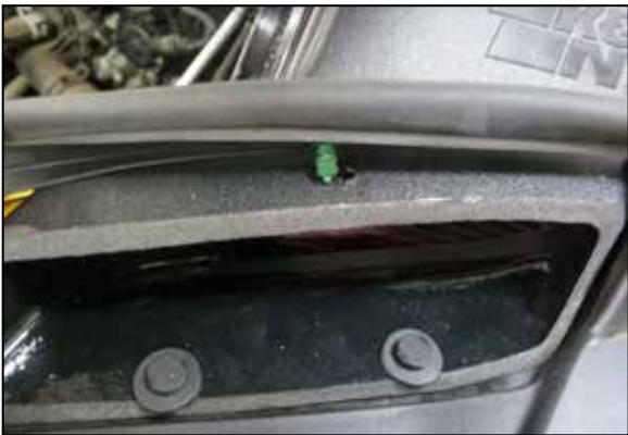
13. Attach the factory hood seal to the fresh air duct of the K&N air filter housing.
