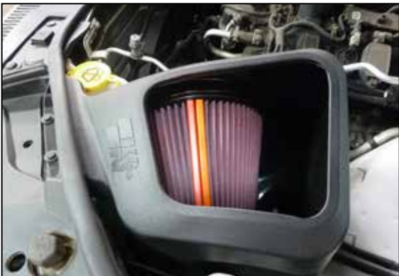
12. Install the K&N air filter housing assembly into the vehicle so the mounting studs insert into the grommets.
