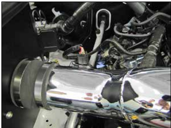
20. Reconnect the mass air sensor electrical connection.
