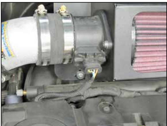
14. Reconnect the mass air sensor electrical connection.
