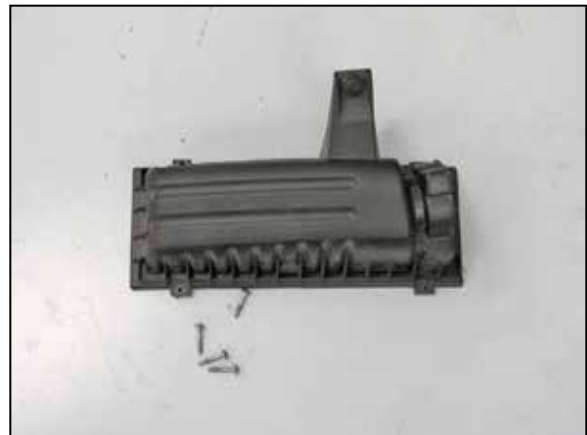
10. Remove the four upper housing mounting screws. NOTE: The screws should be unthreaded from the housing.
