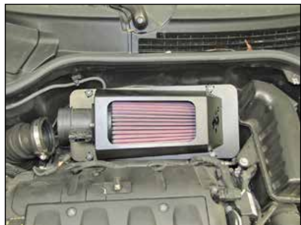
11. Install the K&N® filter assembly onto the lower air filter housing and secure with the factory screws from step #10.
