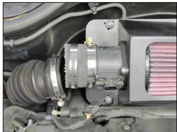
12. Install the silicone hose (08440) onto the throttle body and secure with the provided hose clamp.
