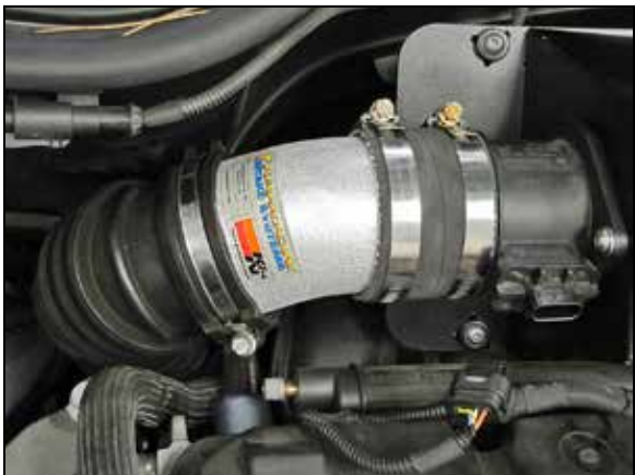
13. Install the K&N® intake tube into the factory hose and then into the hose at the throttle body, then secure with the factory and provided hose clamps.
