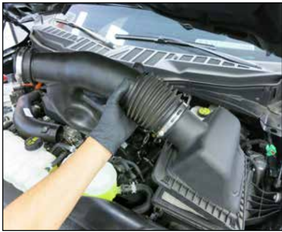
5. Lift the upper air filter housing and intake tube up and out of the engine compartment.
