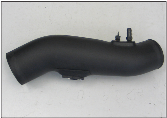
24. Install the provided NPT vent fittings into the K&N® intake tube as shown. NOTE: Plastic NPT fittings are easy to cross thread. Install the vent fitting “hand” tight, then turn it two complete turns with a wrench.
