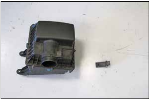
19. Remove the mass air sensor from the factory air filter housing.
