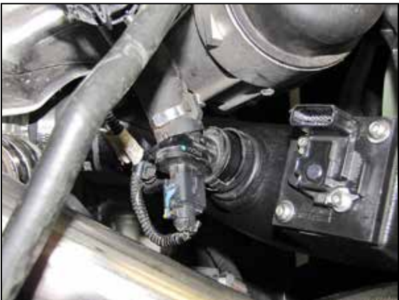
24. Connect the vent Quick disconnect fitting onto the fitting installed into the K&N® intake tube.
