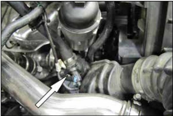
8. Pull the intake tube forward and then disconnect the vent tube quick disconnect and then remove the intake tube from the vehicle.
