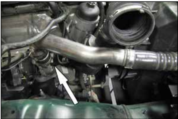
7. Loosen the hose clamp that secures the intake tube to the turbo inlet.
