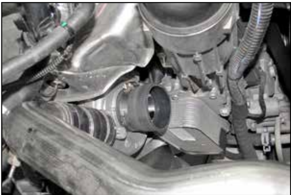
10. Install the coupler hose (08476) onto the turbo inlet and secure with the provided hose clamp.
