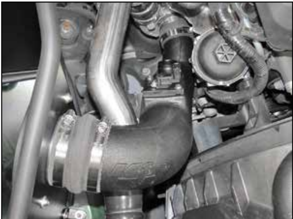
23. Install the K&N® intake tube into the coupler at the turbo and then into the coupler at the filter adapter, adjust the tube for best fit and then secure with the provided hose clamps.
