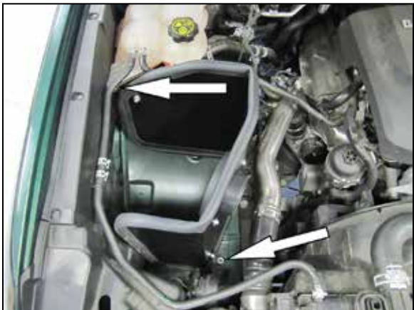
16. Install the heat shield and secure with the factory nut from the previous step and the hardware provided.
