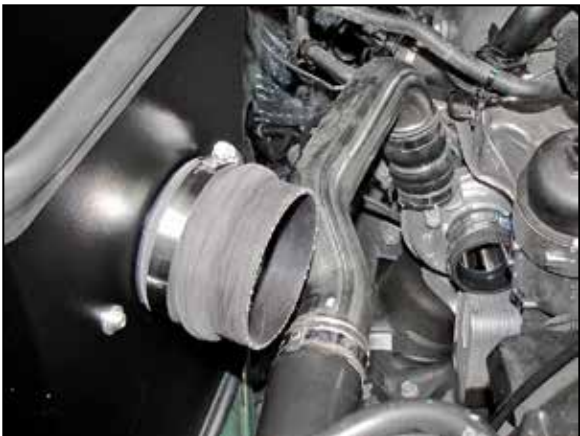
22. Install the provided hump coupler (08699) onto the filter adapter and secure with the provided hose clamp.
