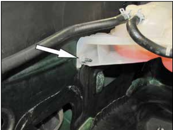
15. Remove the nut shown that secures the coolant reservoir. NOTE: This nut will be reused in the next step.
