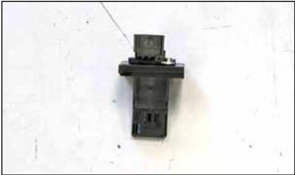
20. Install the mass air sensor into the K&N mass air sensor adapter and secure with the provided hardware.
