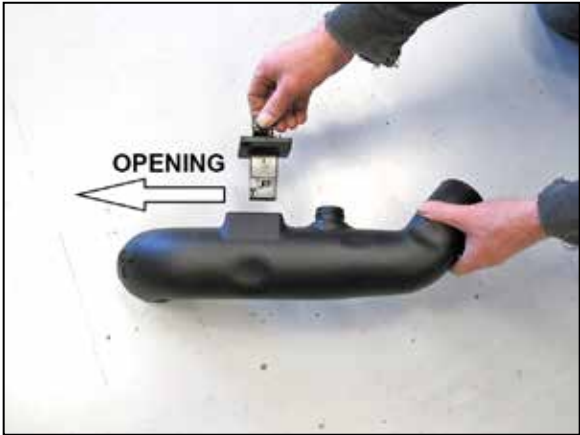
21. Install the mass air sensor assembly into the K&N intake tube so that the opening is towards the filter.
