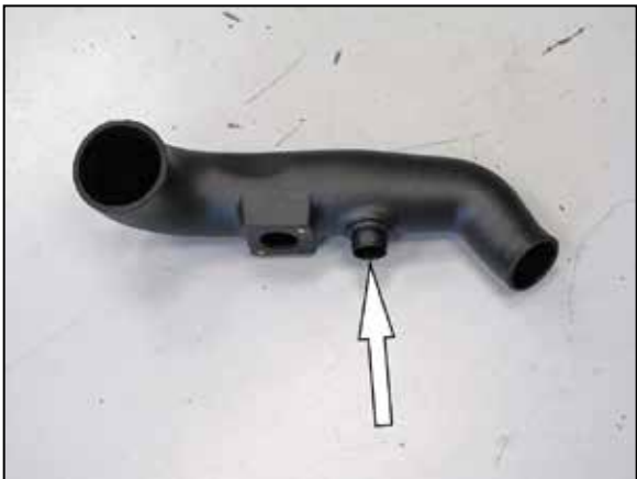
17. Install the provided grommet and quick disconnect fitting into the K&N intake tube.
