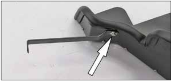
16. Install the heat shield mounting bracket (083103-1) onto the heat shield using the provided hardware. NOTE: Do not completely tighten at this time. NOTE: When using the cut out heat shield wall, place the provided spacer between the bracket and heat shield and use the longer bolt.
