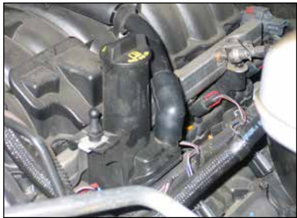
10. Install the crank case vent assembly onto the valve cover port.
