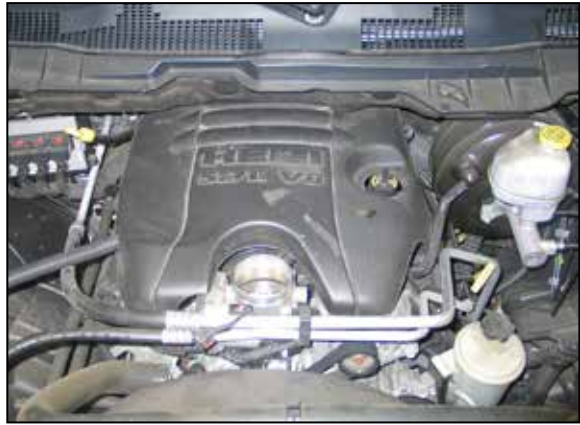
11. Reinstall the engine cover onto the mounting studs and route the crank case vent hose through the opening.
