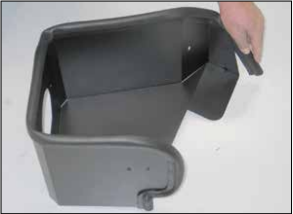
12. Install the provided edge trim onto the heat shield as shown. NOTE: Some trimming of the edge trim will be necessary.
