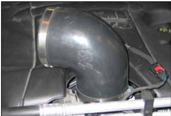
20. Install the provided silicone hose (084086) onto the throttle body and secure with the provided hose clamp.
