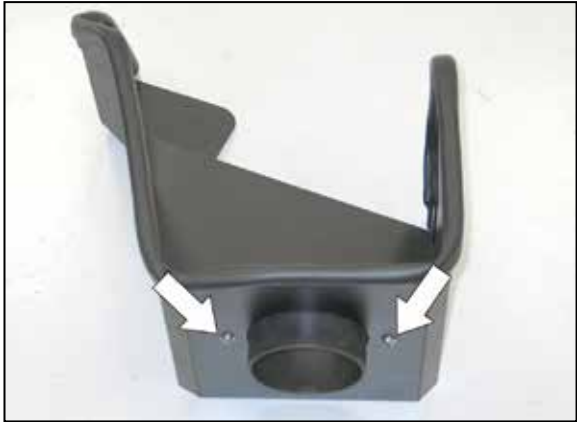
13. Install the provided filter adapter onto the heat shield as shown and secure with the provided hardware.
