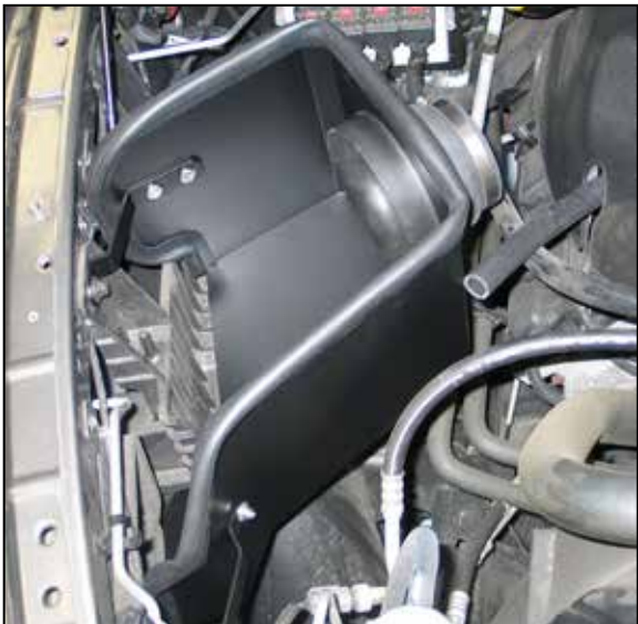
19. Install the heat shield assembly into the vehicle and secure with the bolts removed in steps #17 and 18. Do not completely tighten at this time.
