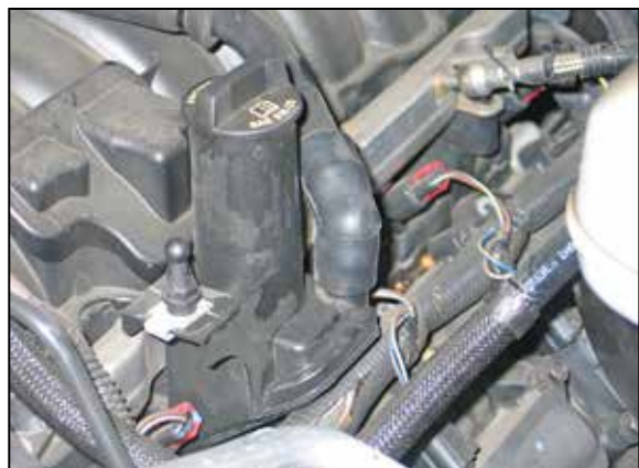
7. Disconnect the crank case vent hose from the valve cover port.
