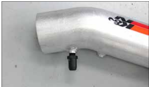
24. Install the 5/8 vent fitting into the K&N® intake tube as shown. NOTE: Plastic NPT fittings are easy to cross thread. Install the vent fitting “hand” tight, then turn it two complete turns with a wrench.
