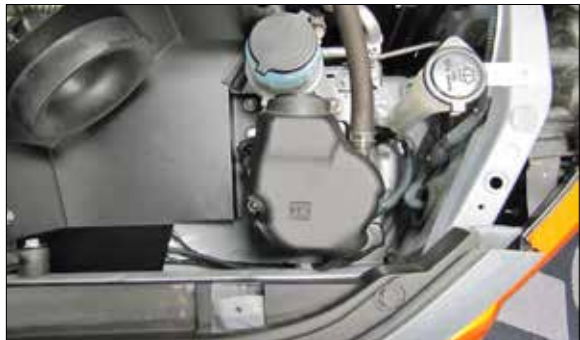
19a. Install the air injection pump onto the heat shield and forward rubber mounted stud and then secure with the provided hardware. Reconnect the air injection pump electrical connection.
