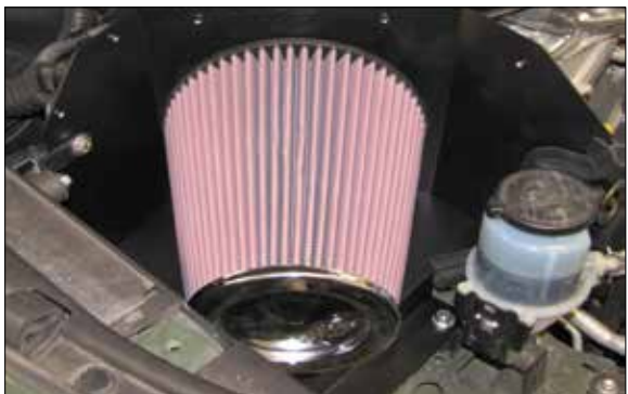
29. Install the K&N® air filter onto the filter adapter and secure with the provided hose clamp. NOTE: Drycharger® air filter wrap; part # RF-1020DK is available to purchase separately. To learn more about Drycharger® filter wraps or look up color availability please visit http://www.knfilters.com ®.
