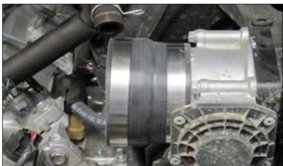
21. Install the provided silicone step hose (084091) onto the throttle body and secure with the provided hose clamp.
