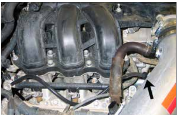
28. Connect the provided fuel pressure vent line to the fuel pressure regulator and then connect the open end to the 3/16 vent fitting in the K&N® intake tube.
