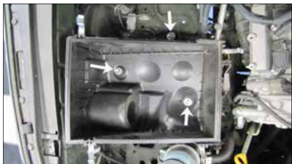
9. Loosen and remove the three bolts securing the lower air box and then remove the lower air box from the vehicle. NOTE: K&N Engineering, Inc., recommends that customers do not discard factory air intake.
