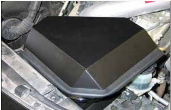
31. Install the heat shield cover onto the heat shield and secure with the provided hardware. NOTE: Use of the heat shield cover is not mandatory; it is recommended that the cover is used during conditions of heavy moisture such as water crossings where water can be thrown from the engine fan.
