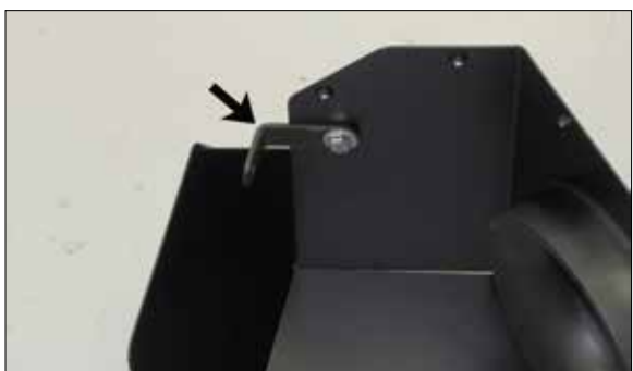
16. Install the provided mounting bracket (08022) onto the heat shield and secure with the provided hardware.
