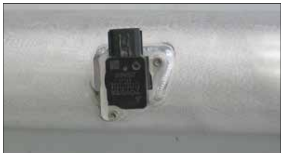
23. Install the mass air sensor into the K&N® intake tube and secure with the provided hardware.
