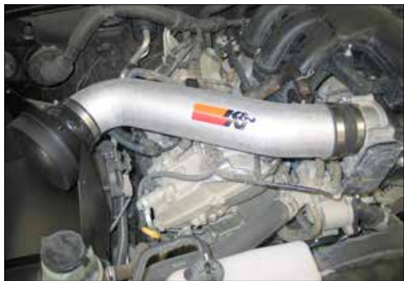
26. Install the K&N® intake tube into hump hose at the filter adapter and then into the silicone hose at the throttle body, align the tube for proper fit and then tighten the hose clamps.
