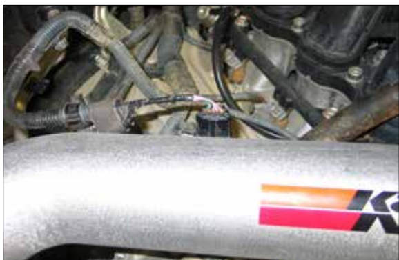
33. Reconnect the mass air sensor electrical connection.
