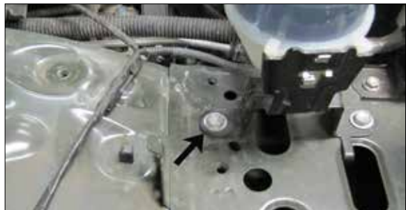
10. Remove the rear P/S reservoir mounting bolt shown.
