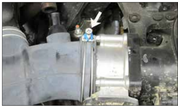
7. Loosen the hose clamp which secures the intake tube to the throttle body.
