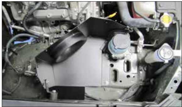
19. Set the heat shield onto the rubber mounted studs and the secure with the provided hardware. NOTE: On models that had a horn attached in this location, be sure to reattach the horn between the heat shield bracket and rubber mounted stud.
