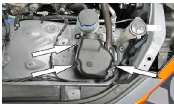
11. On models with the Air injection pump located in front of the air box next to the Power steering reservoir, remove the three bolts securing the pump to the inner fender.
