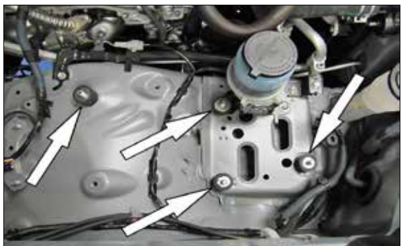
12. Install the four rubber mounted studs into the factory air box and P/S reservoir as shown. NOTE: The forward most rubber mounted stud is only used if the vehicle is equipped with the air injection pump located in front of the factory air box.
