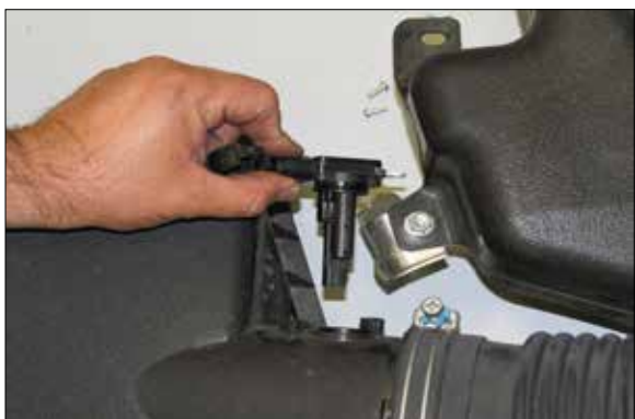
22. Remove the screws which secure the mass air sensor to the factory air box and then remove the mass air sensor from the air box.
