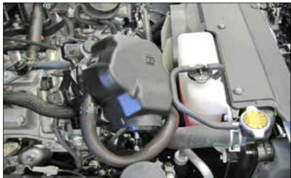
11a. Lift up the air injection pump, disconnect the electrical connection and then set the air injection pump over to side.
