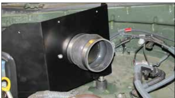
20. Install the provided silicone hump hose (084057) onto the filter adapter and secure with the provided hose clamp.
