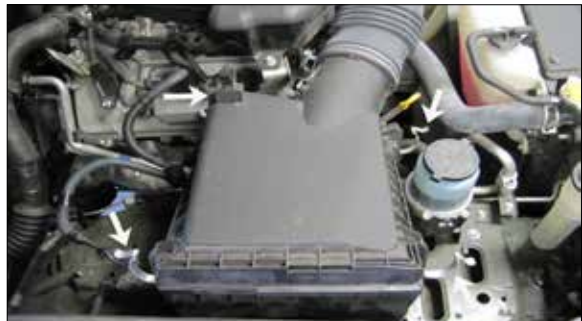
8. Release the four clips which secure the upper air box to the lower air box and then remove the intake tube and upper air box from the vehicle.
