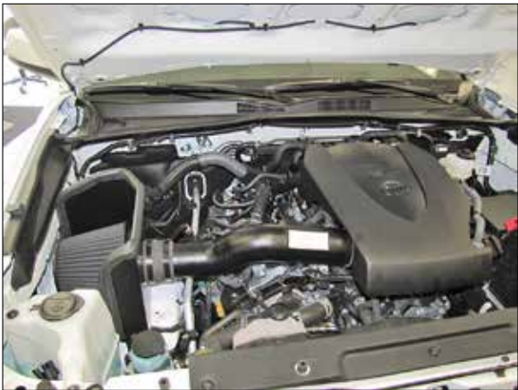
23. Reconnect the vehicle’s negative battery cable. Double check to make sure everything is tight and properly positioned before starting the vehicle.
