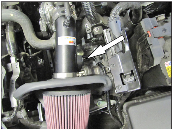
24. Reconnect the mass air sensor electrical connection.
