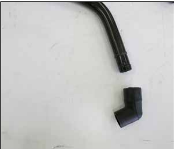
7. Remove the elbow from the plastic hardline.
