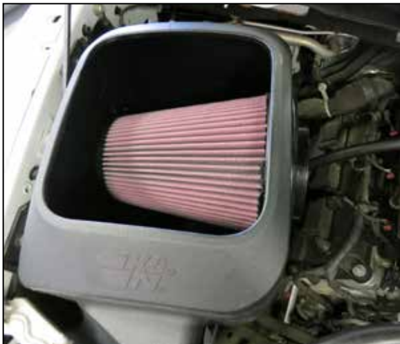
12. Install the K&N air filter into the air filter housing.
