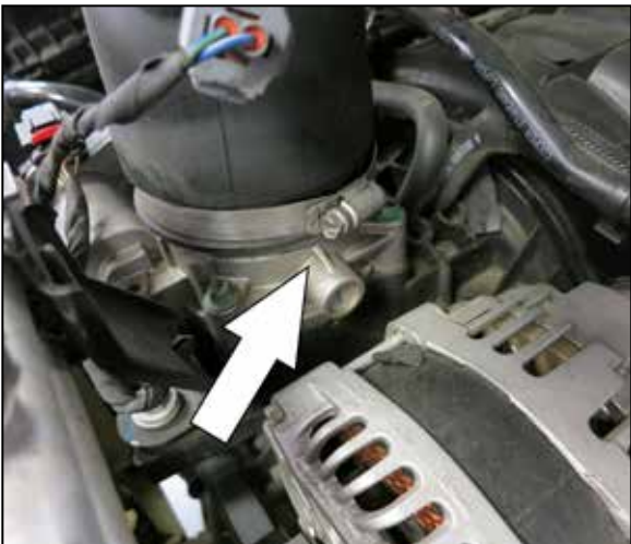
4. Loosen the hose clamp that secures the intake tube to the throttle body.
