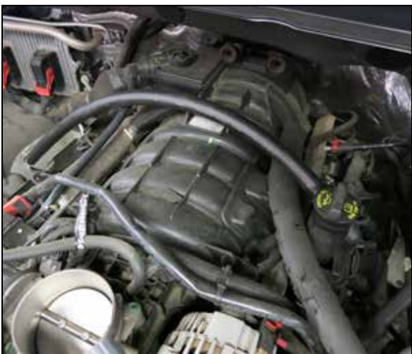
9. Install the CCV hose assembly onto the valve cover port.
