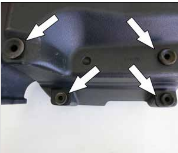
10. Remove the four mounting grommets from the factory air filter housing and install them into the K&N air filter housing as shown.
