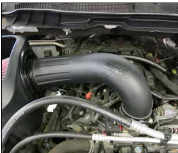
15. Install the K&N intake tube into the air filter and then onto the throttle body, adjust the tube for best fit and then secure the hose clamps.
