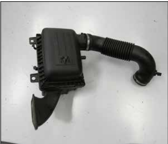
5. Disconnect the intake tube, lift the air filter housing and remove the complete intake system from the Vehicle.
