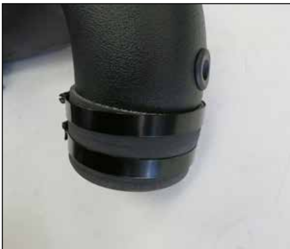
14. Install the provided IAT grommet and coupler hose with clamps.
