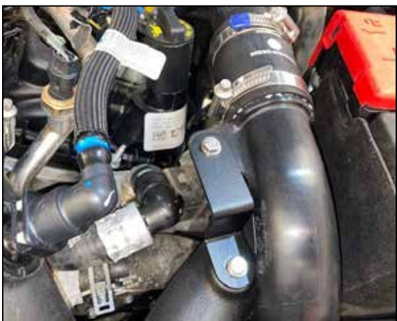
23. Install the provided "Z" bracket to the hot-side charge tube and K&N driver side intake tube and secure with the provided hardware.
