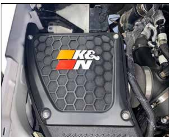
28. Assemble the filter top and then install the assembly on top of the air filter housing and secure with the provided hardware.
