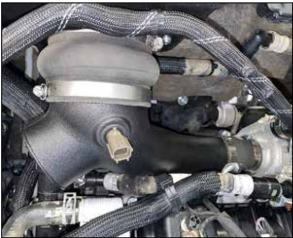
18. Install the K&N intake tube into the coupler at the turbo inlet and then into the coupler at the filter adapter and secure with the provided hose clamps.
