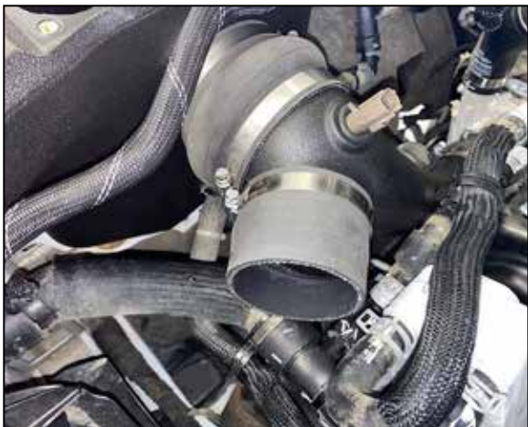
19. Install the remaining straight coupler onto the K&N intake tube and secure with the provided hose clamp.
