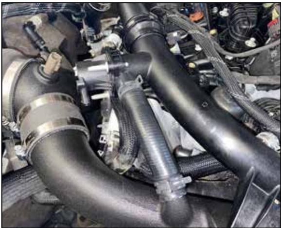
24. Install the BOV hose onto the fitting on the K&N intake tube and secure with the provided spring clamp.
