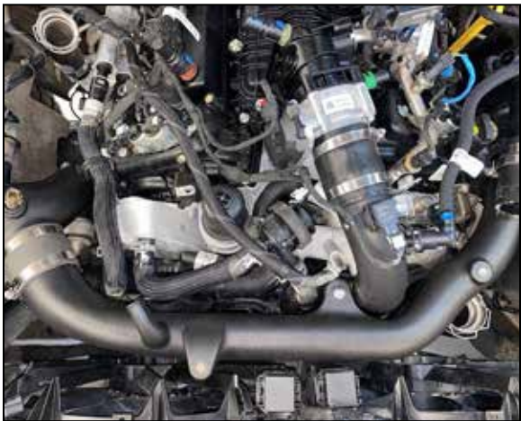
20. Install the driver side K&N intake tube into the factory turbo inlet coupler and then into the coupler on the passenger side K&N intake tube, adjust the tube for best fit and secure with the hose clamps and bolt.
