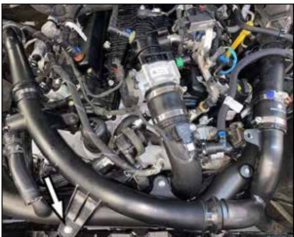
22. Reinstall the factory hot-side charge tube and secure the three connections. Reinstall the factory mounting bolt that secures the tube to the core support.
