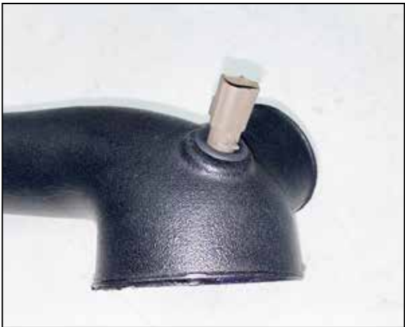
17. Remove the IAT sensor from the factory intake tube, remove the O-ring from the sensor and then install it into the K&N intake tube using the provided grommet. NOTE: The IAT sensor is very fragile, use care while handling the sensor so as not to damage it.
