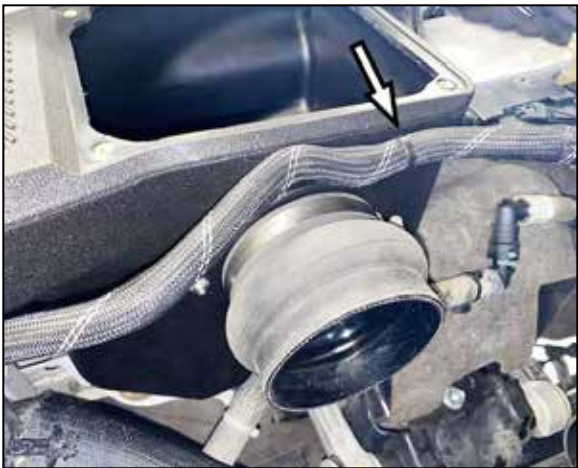
16. Install the provided hump coupler onto the filter adapter and secure with the provided hose clamp. Then secure the upper coolant hose to the air filter housing as shown.
