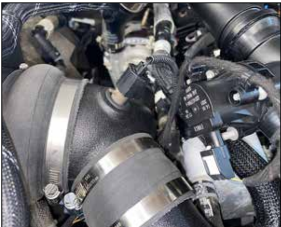
25. Reconnect the IAT sensor and BOV electrical connections and secure the BOV harness to the stud.
