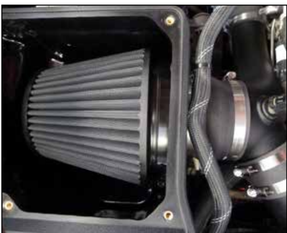
27. Install the K&N air filter onto the filter adapter and secure with the provided hose clamp.
