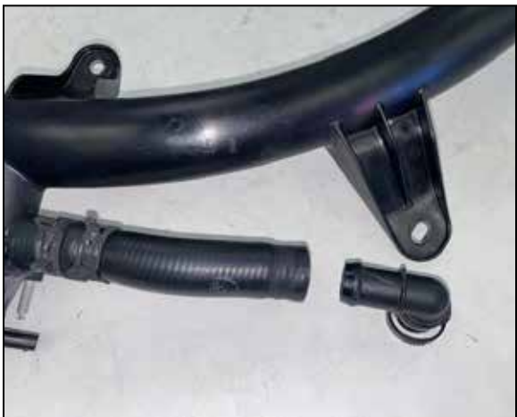
21. Release the spring clamp the secures the quick connect fitting onto the BOV hose and then remove the fitting from the hose.
