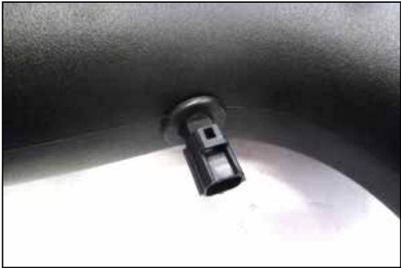
18. With provided grommet, attach to the hole on the intake tube. Install the temperature sensor into the grommet. NOTE: Remove the o-ring for easier installation.
