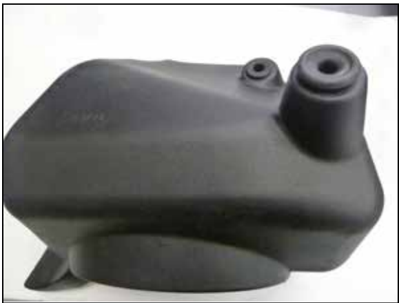
12. Install the 3 grommets from step 10 into the new K&N airbox.
