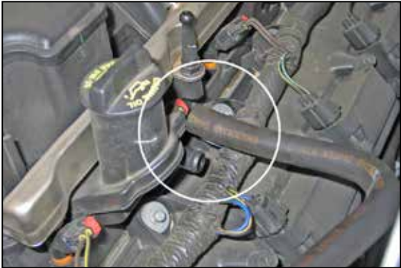
5. Disconnect the crankcase vent hose from the port on the valve cover.
