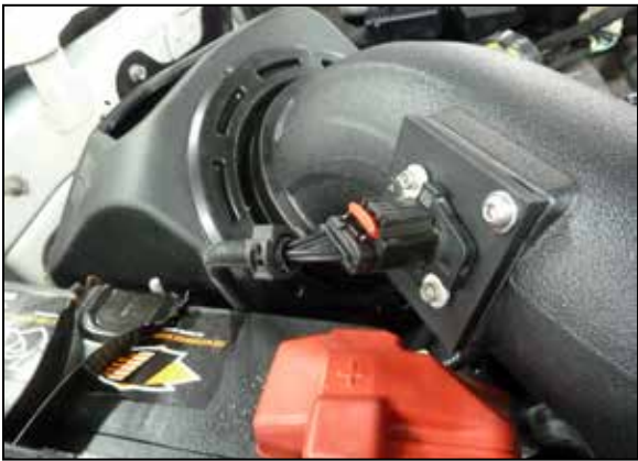
14. Reconnect the mass air sensor using the provided extension harness.
