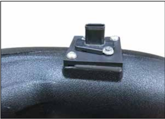
10. Loosen and remove the 2 screws, Install the MAF sensor and secure and tighten. NOTE: Make sure the sensor is going in the correct direction. If it is not installed in the correct orientation, remove the adapter bolts and spin 180 degrees then reinstall the bolts.
