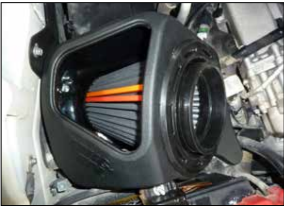
7. Install the K&N filter into the filter housing as shown.
