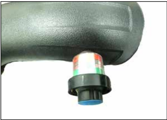
11. Install the filter minder into the K&N intake tube using the provided grommet. NOTE: Pre-assembled from the factory.
