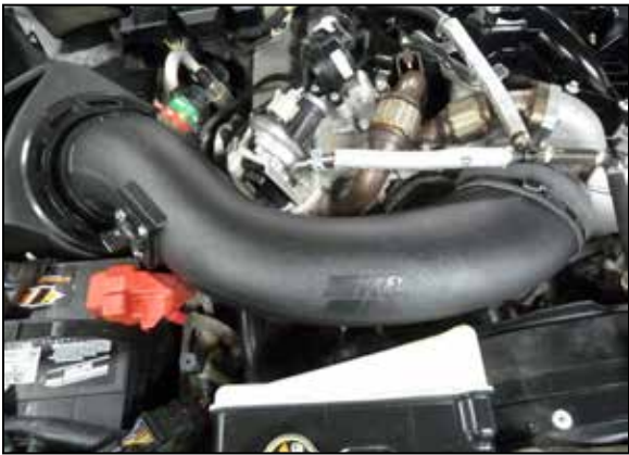
13. Install the intake tube into the filter, align with the turbo inlet, then slide the coupler onto the turbo inlet. Adjust the assembly for best fit and then secure all the hose clamps.
