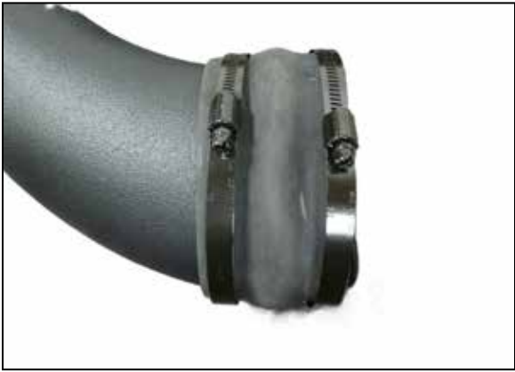
12. NOTE: Pre-assembled from the factory. Install the provided hump coupler and hose clamps onto the K&N intake tube. NOTE: Slide the coupler all the way onto the intake tube and do not secure the hose clamps.
