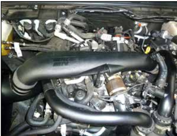
25. Install the K&N driver side intake tube into the factory turbo inlet fitting and then into the coupler at the passenger side intake tube, adjust the tube for best fit and then secure with the hose clamps. Tighten clamps using 5/16" socket or nut driver. NOTE: Do not over tighten clamps.
