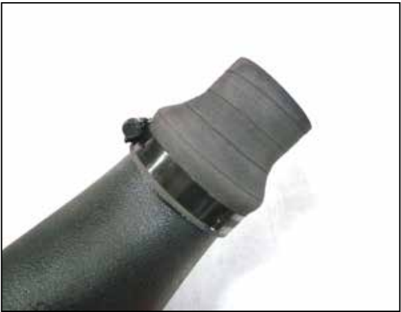
19. Install the reducer coupler onto the K&N passenger side intake tube and secure with the provided hose clamp. Tighten clamp using 5/16" socket or nut driver. NOTE: Do not over tighten clamps.
