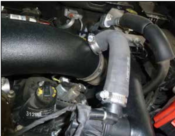
27. Install the provided BOV hose onto the valve and K&N intake tube and secure with the provided hose clamps. Tighten clamps using 5/16" socket or nut driver. NOTE: Do not over tighten clamps.
