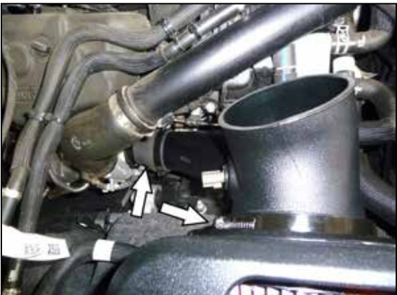
20. Install the K&N passenger side intake tube onto the turbo and then into the K&N air filter, adjust the tube for best fit and then secure with the provided hose clamps. Tighten clamps using 5/16" socket or nut driver. NOTE: Do not over tighten clamps.
