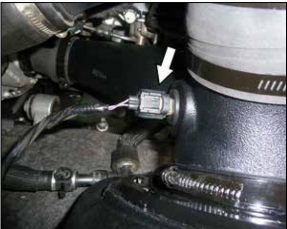
22. Connect the IAT sensor electrical connection.
