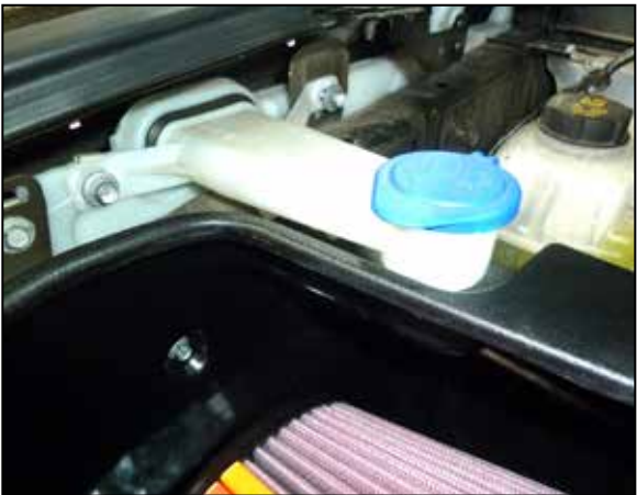
17. Reinstall the washer bottle filler neck and secure with the factory mounting bolts removed during step #11.
