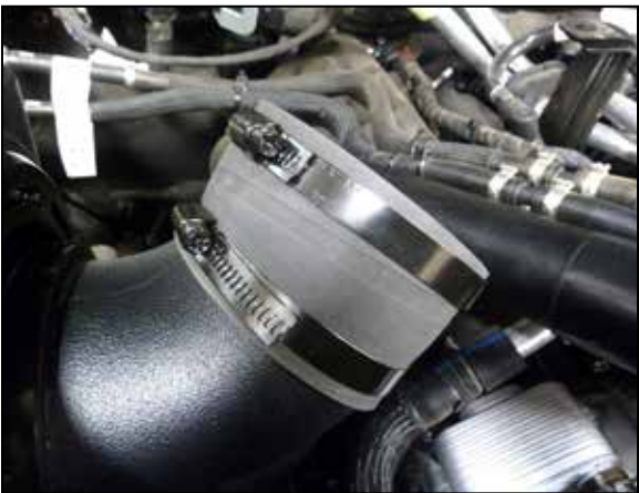
21. Install the provided coupler onto the open end of the passenger side intake tube, do not fully secure the hose clamp for the coupler currently. Tighten clamp using 5/16" socket or nut driver. NOTE: Do not over tighten clamps.
