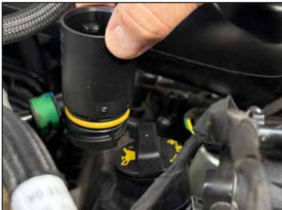
24. On some models, remove the oil filler neck extension and install the oil cap only.
