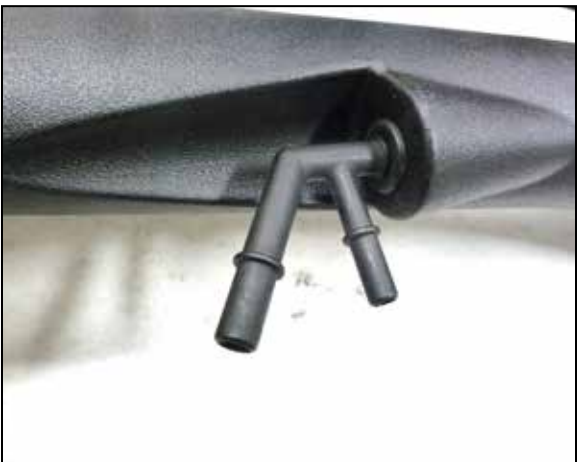
23. Install the K&N ejector fitting into the K&N driver side intake tube using the provided grommet. NOTE: Do not use excessive force with the ejector fitting as it is fragile.
