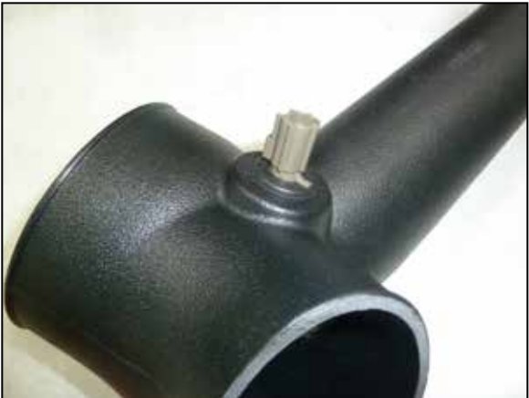
18. Remove the IAT sensor from the factory housing, remove the O-ring from the sensor and then install the sensor into the K&N passenger side intake tube using the provided grommet.
