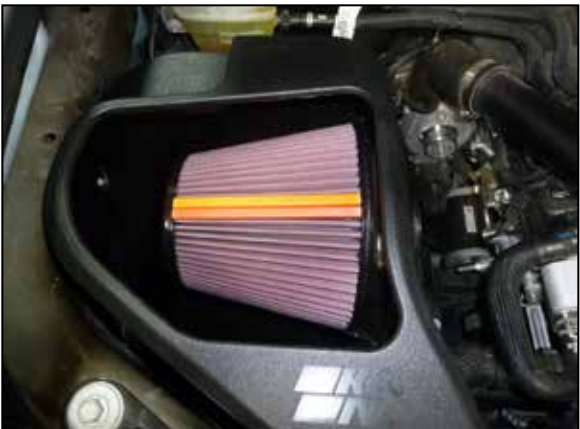
16. Install the K&N air filter into the K&N air filter housing.
