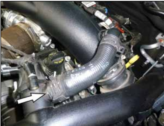
26. Release the spring clamp that secures BOV hose to the valve and then remove the hose from the vehicle.
