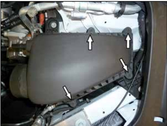
7. Remove the four bolts that secure the upper air filter housing and then remove the upper housing from the vehicle.
