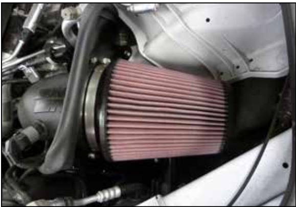
21. Install the K&N air filter onto the intake tube and secure with the provided hose clamp.
