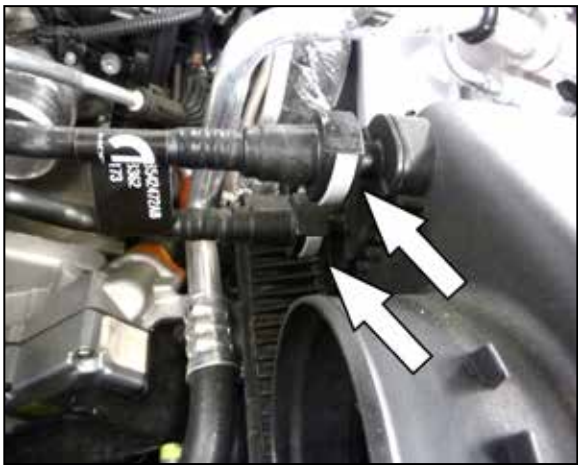
6. Push in the locking tabs and then disconnect the Ejector lines from the intake plenum.
