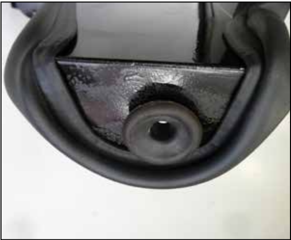
10. Remove the factory air filter housing mounting grommet and then install it into the K&N heat shield as shown.
