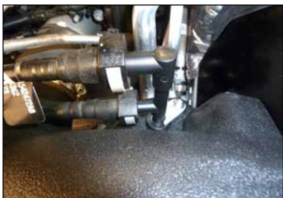
17. Connect the Ejector vent lines to the K&N Ejector F-fitting.
