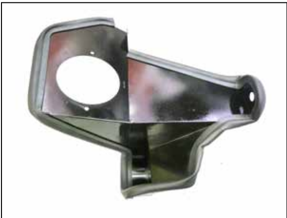
9. Install the provided edge trim onto the heat shield as shown. Some trimming of the edge trim will be necessary.
