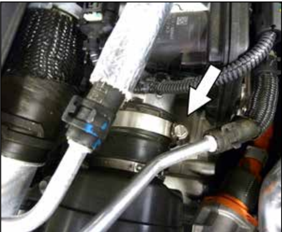
5. Loosen the hose clamp the secures the intake hose to the turbo inlet and then remove the hose from the vehicle.
