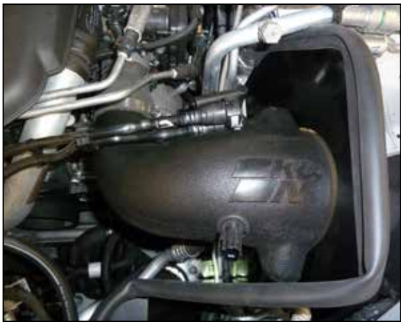
15. Install the K&N intake tube into the heat shield and coupler.
