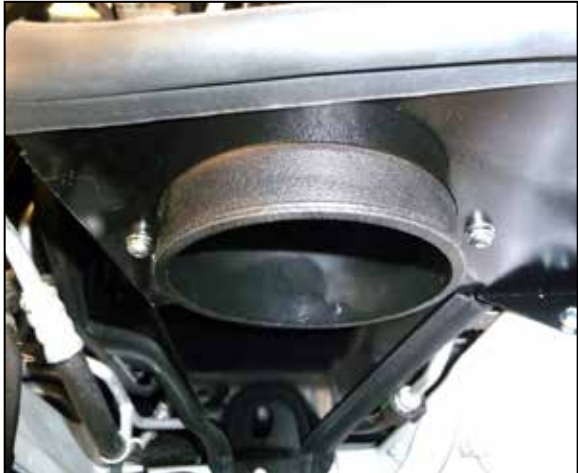
16. Secure the tube to the heat shield with the provided hardware and tighten the hose clamp at the coupler.
