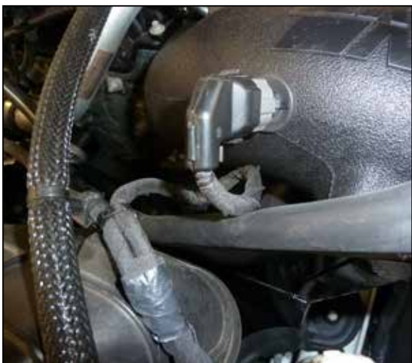
19. Reconnect the IAT sensor electrical connection.
