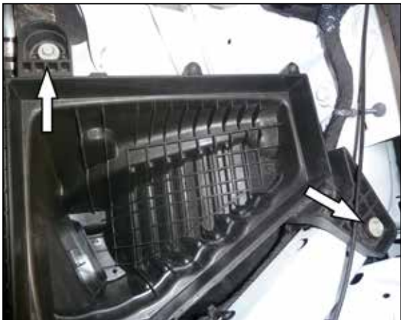
8. Remove the two bolts that secure the lower air filter housing and then remove the housing from the vehicle.
