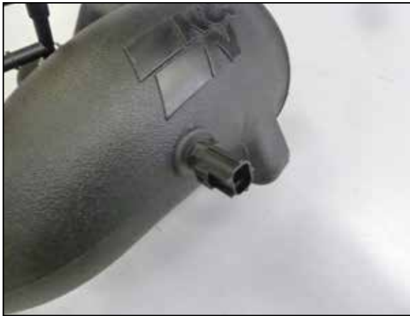
14. Remove the IAT sensor from the factory intake hose and install it into the K&N intake tube with the provided grommet.
