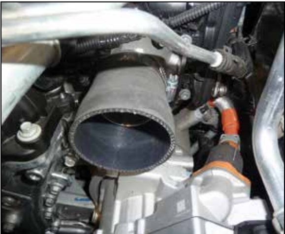
12. Install the step coupler onto the turbo inlet and secure with the provided hose clamp.
