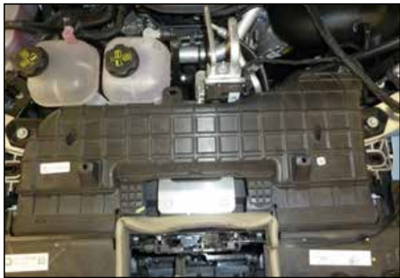
18. Reinstall the fresh air duct and secure with the factory hardware.
