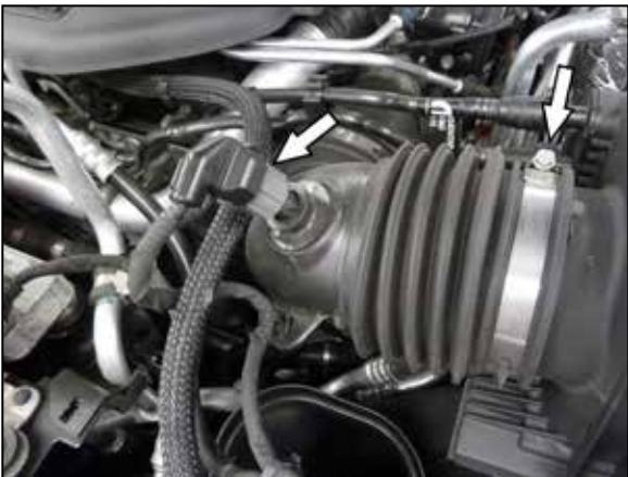
4. Disconnect the IAT sensor electrical connection. Loosen the hose clamp that secures the intake hose to the air filter housing.
