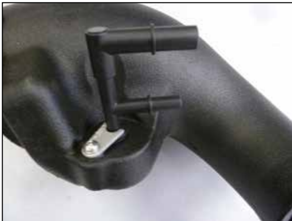
13. Install the provided O-ring onto the K&N Ejector fitting then install the fitting into the K&N intake tube and secure with the provided mounting clip and hardware.
