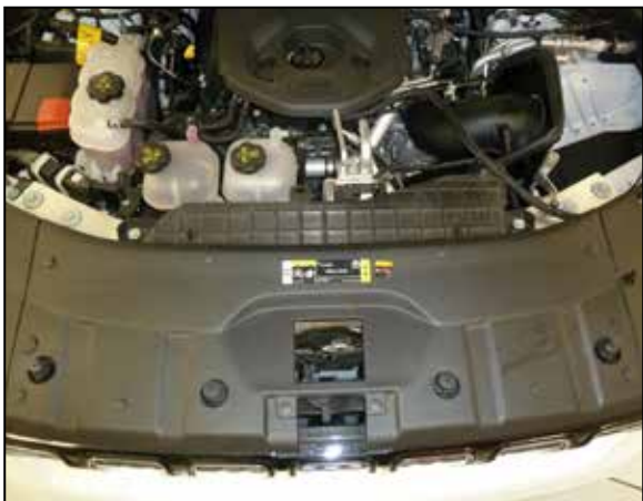
20. Reinstall the valence and secure the factory push pins.
