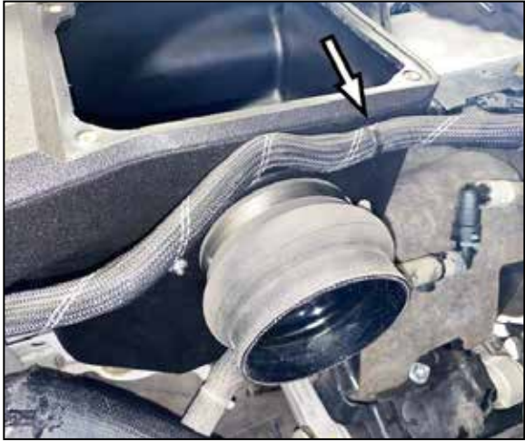
16. Install the provided hump coupler onto the filter adapter and secure with the provided hose clamp. Then secure the upper coolant hose to the air filter housing as shown.
