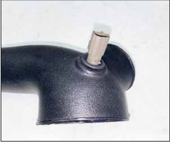
17. Remove the IAT sensor from the factory intake tube, remove the O-ring from the sensor and then install it into the K&N intake tube using the provided grommet. NOTE: The IAT sensor is very fragile, use care while handling the sensor so as not to damage it.
