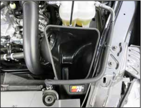
17. Install the K&N air filter housing into the vehicle and secure with the factory bolt from the previous step.
