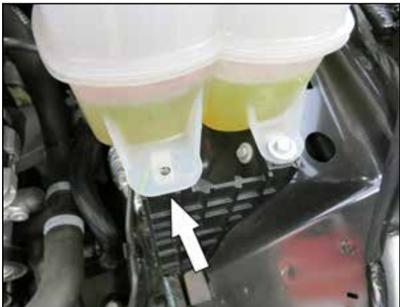
16.Remove the coolant bottle mounting bolt shown.
