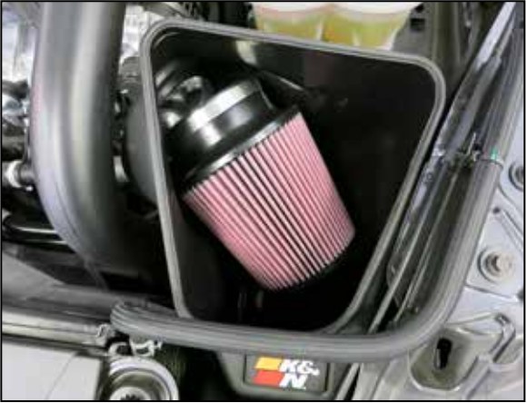
18. Install the K&N air filter into the K&N air filter housing.
