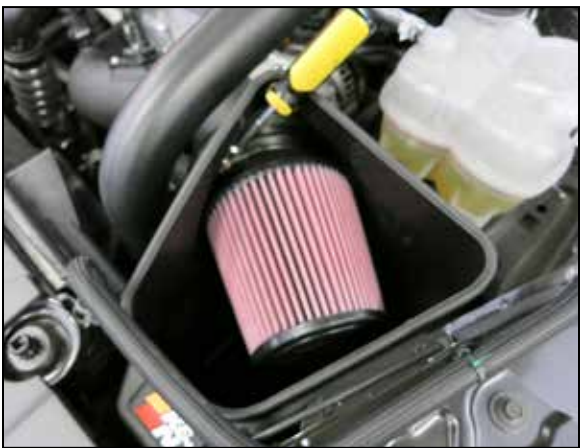
23. Install the air filter onto the intake tube and secure with the provided hose clamp.
