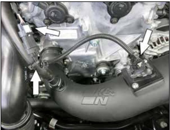
22. Install the provided MAF harness extender and secure with the provided tie wrap.
