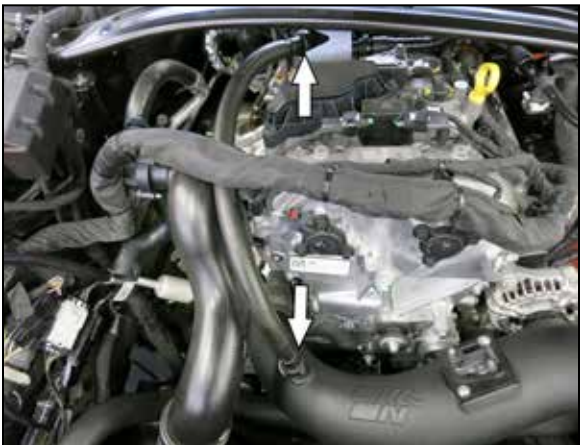
21. Install the CCV hose assembly onto the fittings on the valve cover and intake tube.
