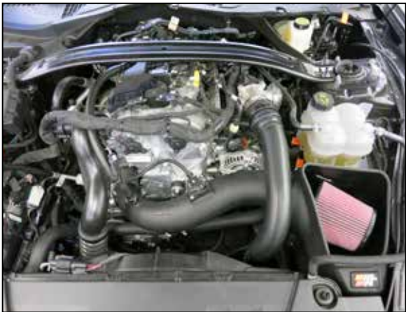
25. Reconnect the vehicle's negative battery cable. Double check to make sure everything is tight and properly positioned before starting the vehicle.
