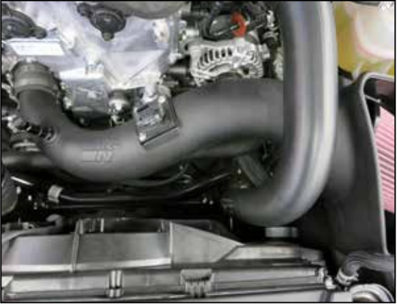
19. Install the intake tube through the seal in the air filter housing and then into the coupler at the turbo. Adjust the tube for best fit and then secure with the provided hose clamps.
