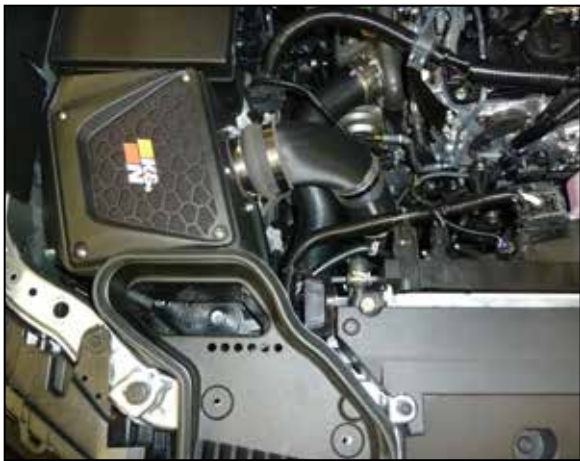
32. Reconnect the vehicle's negative battery cable. Double check to make sure everything is tight and properly positioned before starting the vehicle.
