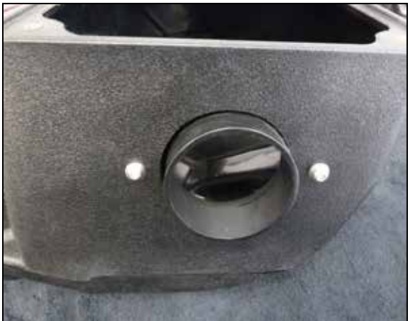
21. Install the filter adapter into the K&N air filter housing and secure with the provided hardware.
