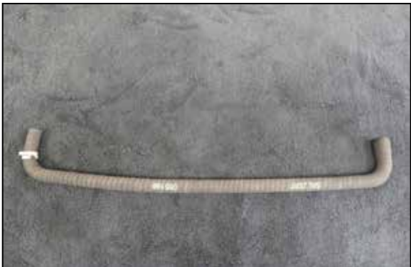
25. Install the factory spring clamp from step #8 onto the small end of the provided vent hose.
