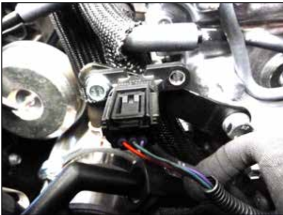
28. Using the provided bracket and hardware, mount the vacuum sensor to the engine as shown and then connect the vacuum line from the tee fitting connected to the ejector fitting. NOTE: The bracket/sensor may have to be rotated or positioned properly allowing the harness to be connected.
