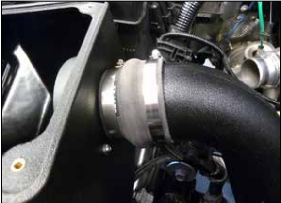
23. Install the provided hump coupler onto the intake tube and filter adapter, align for best fit and then secure with the provided hose clamps.
