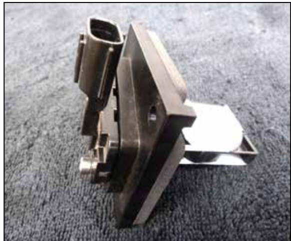
16. Install the gasket onto the K&N maf adapter. Remove the maf sensor from the factory housing and install it into the K&N adapter and secure with the provided hardware.
