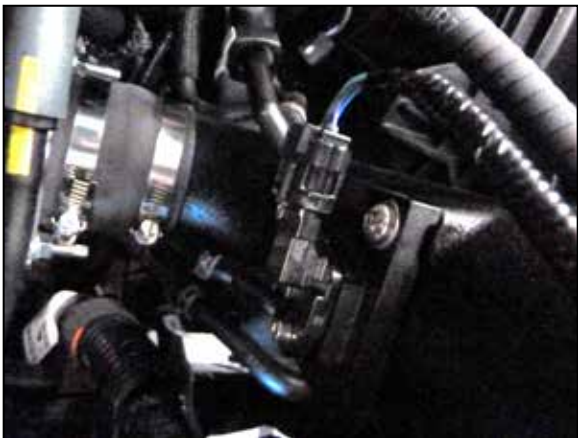
27. Reconnect the MAF sensor electrical connection.
