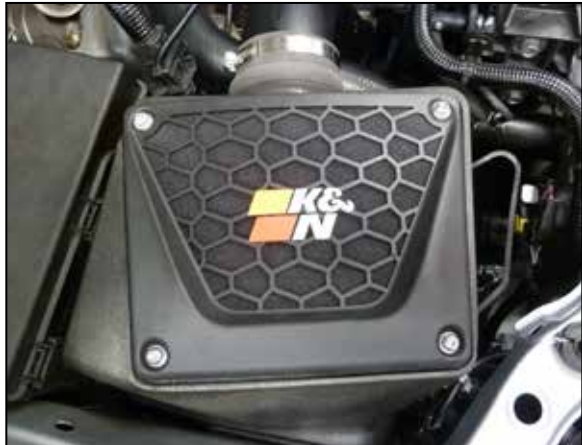
30. Assemble the pre-filter lid and install it onto the K&N air filter housing using the provided hardware.
