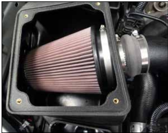
29. Install the K&N air filter onto the filter adapter and secure with the provided hose clamp.
