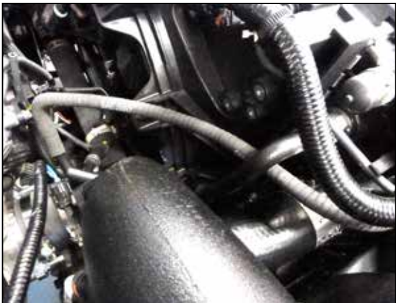
26. Install the vent hose onto the ejector fitting installed into the K&N intake tube and then connect the open end onto the charge tube fitting.
