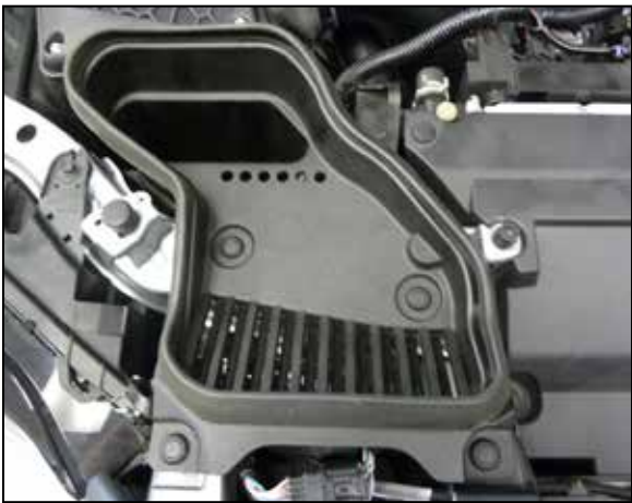
31. Reinstall the factory fresh air duct and secure with the factory pins. NOTE: Land Cruiser models do not use the under hood fresh air duct, skip to the next step.
