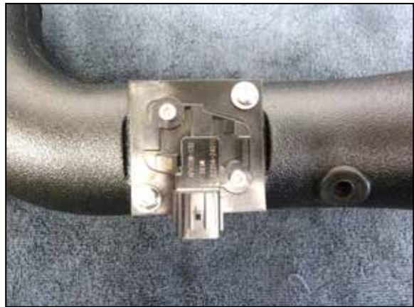
17. Install the maf assembly into the K&N intake tube, be sure to install the assembly in the correct orientation with the opening towards the air filter end of the tube.
