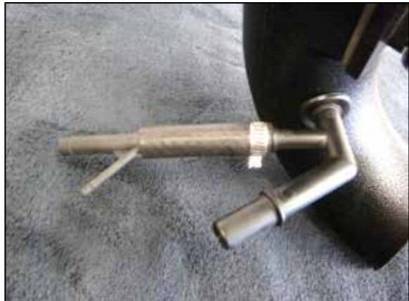
19. Install the Ejector fitting assembly into the K&N intake tube using the provided grommet.
