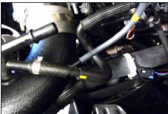
20. Install the intake hose assembly onto the turbo inlet. Connect the vent hoses from step #11 and #12 to the vacuum fitting as shown.
