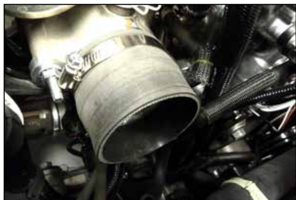
15. Install the provided coupler onto the turbo inlet and secure with the provided hose clamp.
