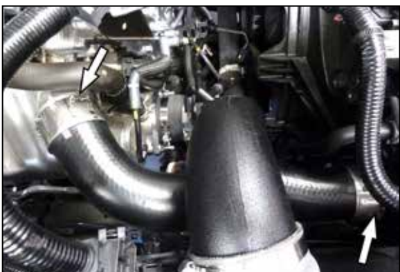
24. Reinstall the charge tube and secure with factory retaining clips.
