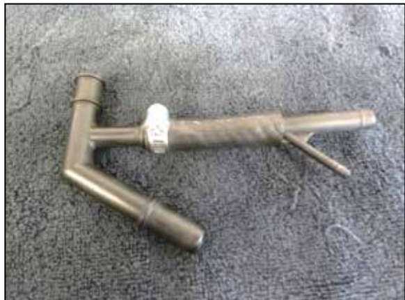
18. Assemble the provided Ejector fitting, vacuum hose & vacuum fitting as shown.
