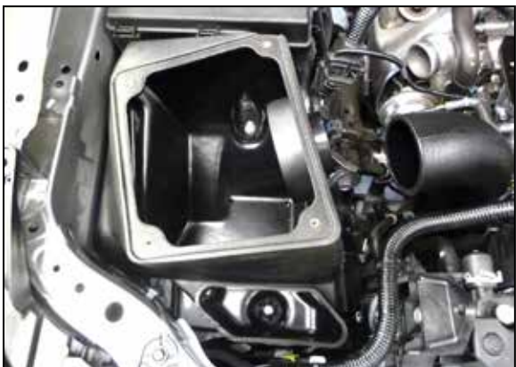
22. Install the K&N air filter housing assembly into the vehicle and secure with the provided hardware. NOTE: On Land Cruiser models, install the provided block-off plug onto the under hood fresh air duct inlet.
