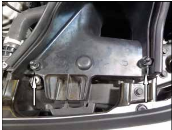
5. Remove the two bolts that secure the fresh air duct to the core support.
