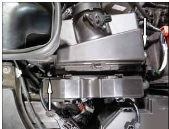
6. Remove the two bolts that secure the air filter hosing and then remove the housing from the vehicle. NOTE: K&N Engineering, Inc., recommends that customers do not discard factory air intake.
