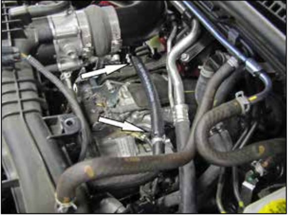
21. Install the K&N® crank case vent hose onto the fitting installed into the intake tube and then connect the union to the factory crank case vent hose.
