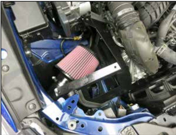
22. Install the mounting posts into the factory air filter housing mounting locations on the inner fender, then install the K&N heat shield onto the posts.
