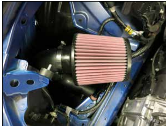
18. Install the K&N air filter onto the intake tube and secure with the provided hose clamp.
