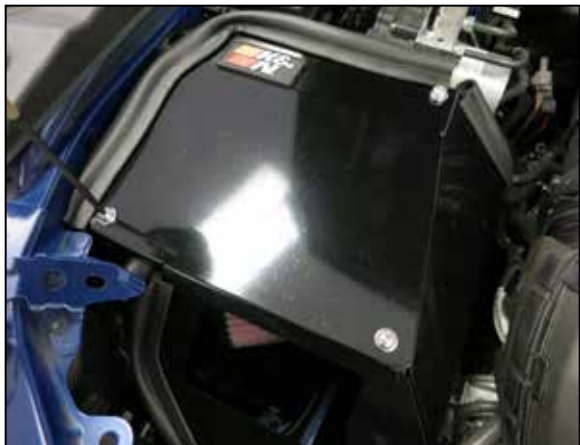
25. Install the lid onto the heat shield and secure with the provided hardware.
