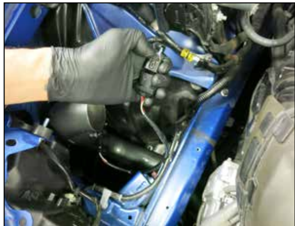
16. Install the K&N intake tube into the coupler at the turbo and align the mounting bracket with the vibration damper. Connect the provided extension harness to the mass air sensor and then connect the other end to the factory harness.
