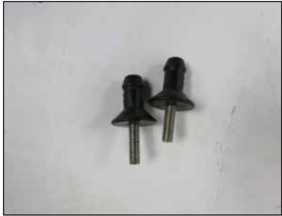
19. Install the provided m6 studs into the provided mounting posts.
