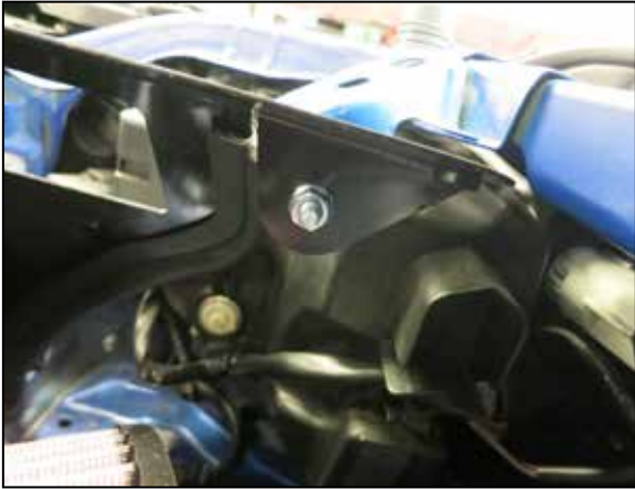
23. Secure the heat shield to the vibration damper using the factory nut.
