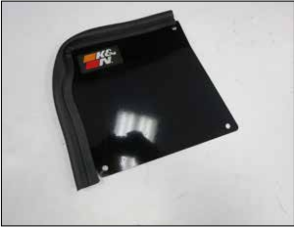
24. Install the remaining 15" edge trim onto the lid as shown. Install the K&N badge and secure with the backing plate.
