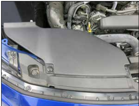
26. Reinstall the fresh air duct and secure with the factory mounting pins.
