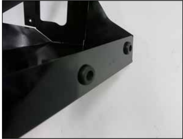
20. Install the provided grommets into the base of the heat shield as shown.
