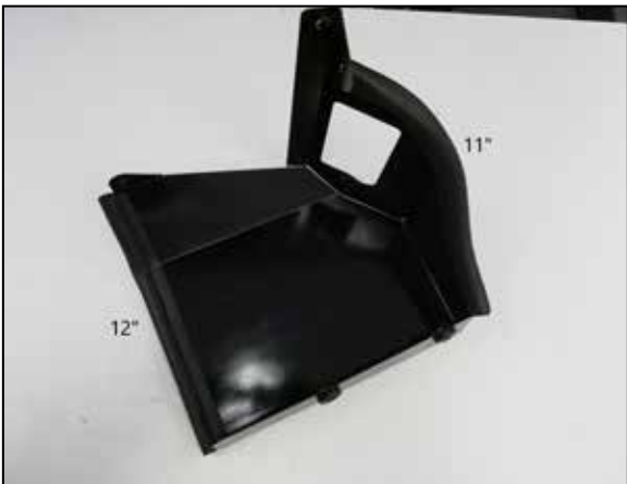
21. Cut the provided edge trim into lengths of 11", 12" and 15". Install the 11" and 12" onto the heat shield as shown.
