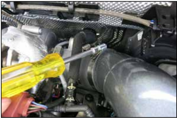
16. Insert the intake tube through the heat shield and into the coupler at the turbo, adjust for best fit and secure with the provided hose clamp.
